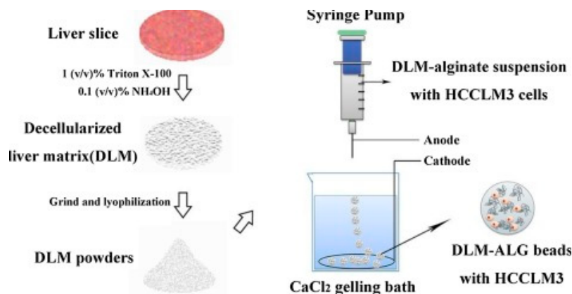
Figure 12. Schematic showing the preparation of decellularized liver matrix (DLM) and DLM-alginate hybrid gel beads (DLM–ALG beads). Reprinted with permission from Elsevier, Sun et al., Int. J. Biol. Macromol. , 2018 [170].
