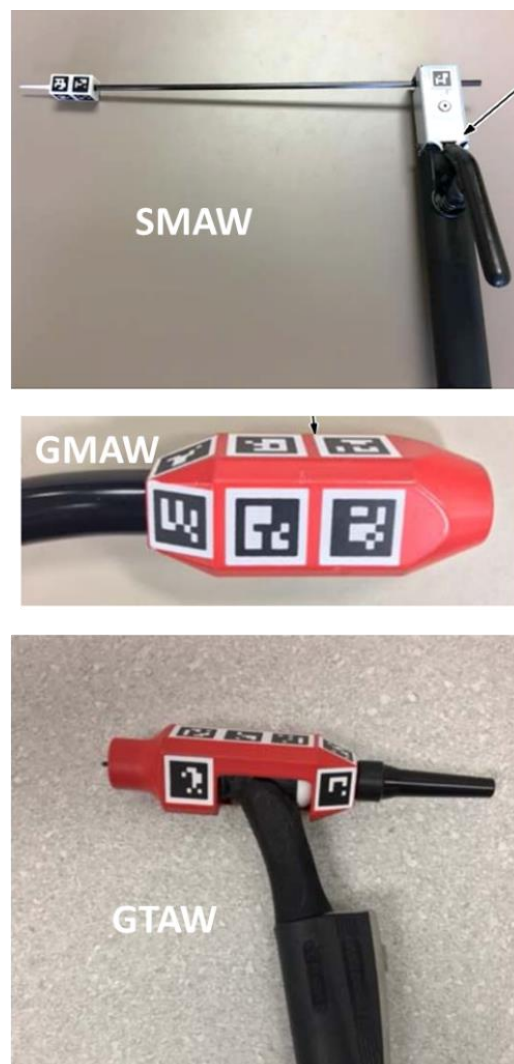
Figure 4: Augmented reality welding torches and electrodes for SMA, GTA ad GMA welding processes
