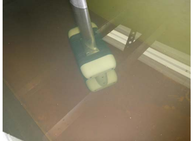
Fig. 5. The 1/4-scale Clio model mounted on the apparatus of Fig. 4, shown at a side-slip angle of 15^\circ . The model can be mounted with either the roll-axis actuated (as shown) or the pitch axis. (The axes refer to the full-scale vehicle.)
