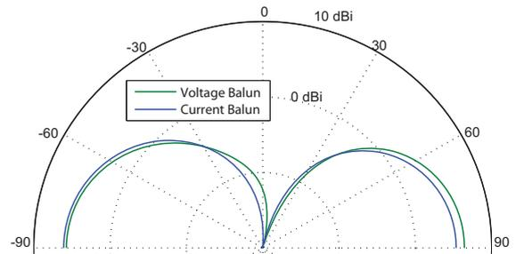
Fig. 15. E-plane pattern of vertically-polarized biconical antenna driven by voltage and current baluns at 55 MHz.
