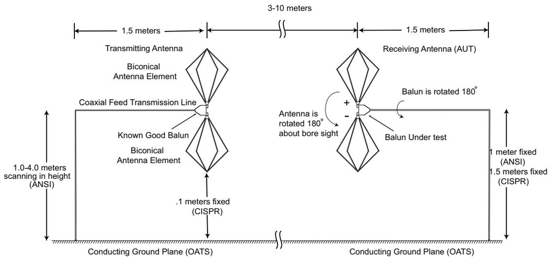
Fig. 1. Balun symmetry test: The antenna on the left is known good and is to be a source of vertically-polarized, quasi-plane wave radiation. In the ANSI standard this antenna is scanned to avoid nulls due to interference between the LOS and ground bounce rays. In some of the original NPL tests, this antenna was a monopole. The inversion is performed by rotating the balun and antenna on the right  $180^\circ$  about its bore-sight axis such that the minus sign is up and the plus sign down.
