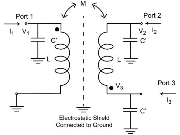
Fig. 18. Faraday transformer with a grounded electrostatic shield between the primary and secondary.
