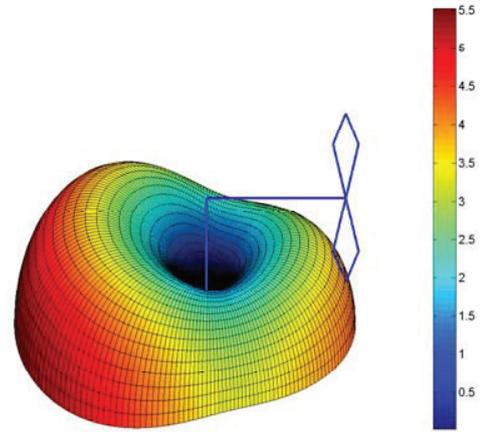
Fig. 14. 3-dimensional radiation pattern depicting the total gain of the vertically-polarized biconical antenna driven by a voltage balun at 60 MHz.
