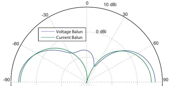
Fig. 11. E-plane pattern of vertically-polarized biconical antenna driven by voltage and current baluns.
