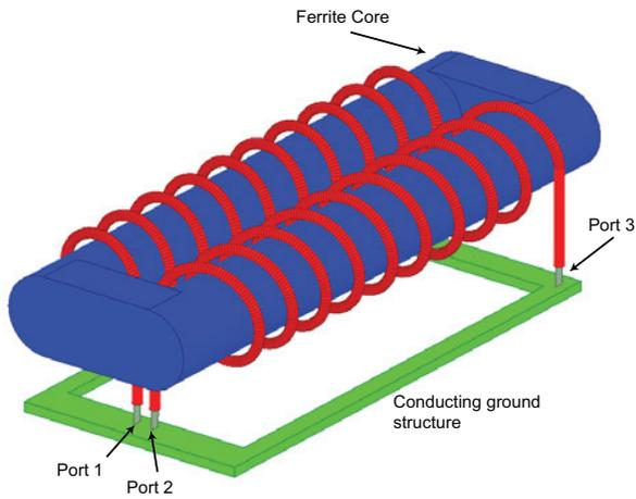
Fig. 19. Simple Faraday transformer with ferrite core. The green conductive frame at the bottom serves as a ground and the three lumped ports in the simulation can be seen connecting the red windings to ground.
