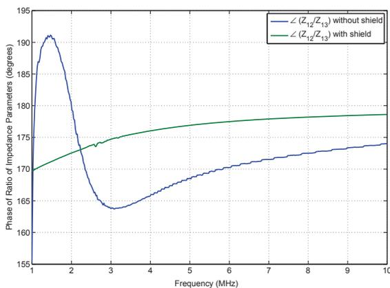
Fig. 23. The phase of the ratio  $\frac{Z_{12}}{Z_{13}}$  with and without the shield. Again, the shield forces this phase much closer to its ideal value of 180°.
