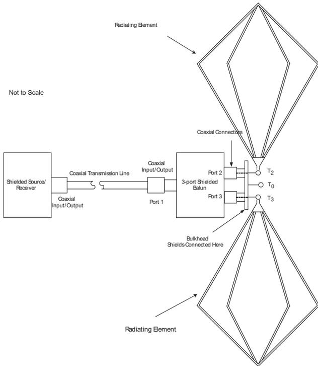
Fig. 2. Biconical antenna driven by 3-port, shielded, “connectorized” balun: The location of the three terminals for a sound physical port representation are indicated by  $T_0$ ,  $T_2$ , and  $T_3$  [11]. Port 2 comprises terminals  $T_2$  and  $T_0$  while port 3 comprises terminals  $T_3$  and  $T_0$ .
