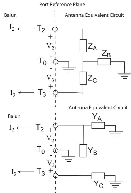
Fig. 3. Equivalent T and  $\Pi$  networks for the terminals shown in Fig. 2. The terminals and ports correspond to those in Fig. 2. The positive current direction for each port is into the port of the balun and thus out of the equivalent network of the antenna.
