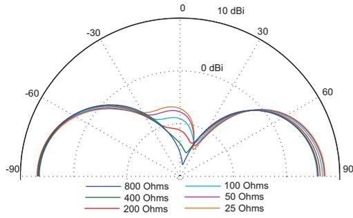
Fig. 12. E-plane pattern of vertically-polarized biconical antenna driven by 180° hybrid with the sum port terminated.
