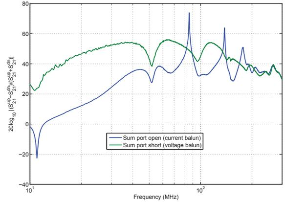
Fig. 8. Eqn 16 from balun inversion test in Fig. 7 as computed with HFSS.
