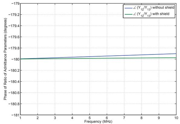
Fig. 21. The phase of the ratio  $\frac{Y_{12}}{Y_{13}}$  with and without the electrostatic shield. Again note the  $y$ -axis scale—the shield changes the phase of the ratio  $\frac{Y_{12}}{Y_{13}}$  by less than  $0.1^\circ$ .
