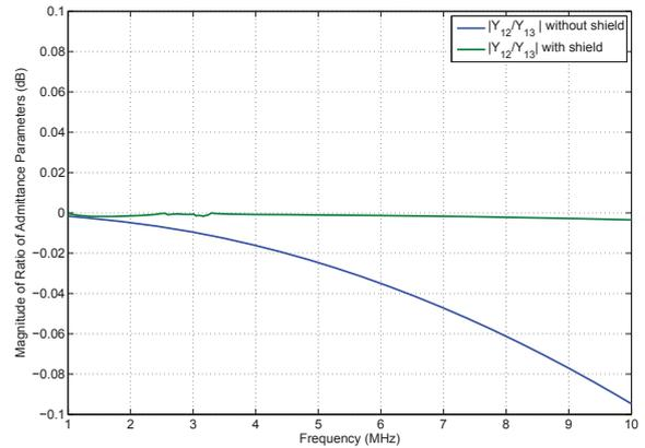
Fig. 20. The magnitude of the ratio  $\frac{Y_{12}}{Y_{13}}$  with and without the electrostatic shield. Note the  $y$ -axis scale—the shield changes the magnitude of the ratio  $\frac{Y_{12}}{Y_{13}}$  by less than 0.1 dB.
