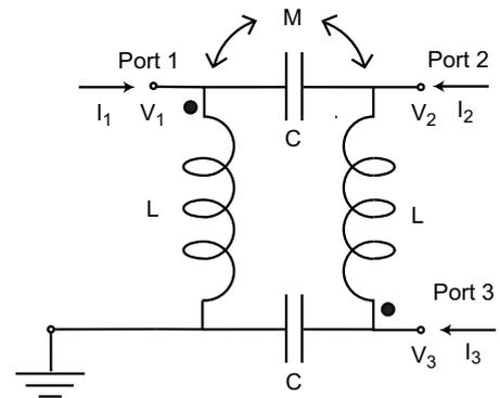
Fig. 17. Faraday transformer with inter-winding capacitance. The dot arrangement or relative sense of the windings corresponds to the numerical example in this section.
