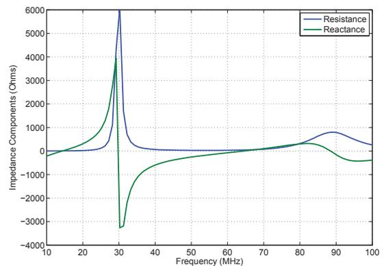
Fig. 16. Common-mode impedance of biconical antenna driven against exterior of feed transmission line.
