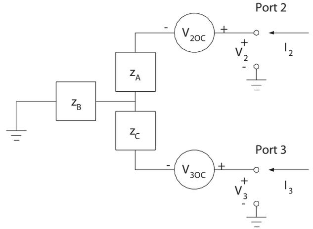
Fig. 10. Thévenin equivalent network for a reciprocal 3-port balun.
