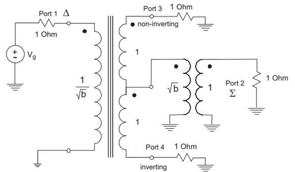
Fig. 6. Lumped hybrid transformer as portrayed in Fig. 4.12 (b) of ref. [15] or Fig 1 of ref. [14].
