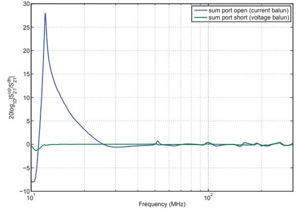
Fig. 7. Ratio of transmission scattering parameters  $\left| \frac{S_{21}^{up}}{S_{21}^{dn}} \right|$  in balun inversion test as computed with HFSS.
