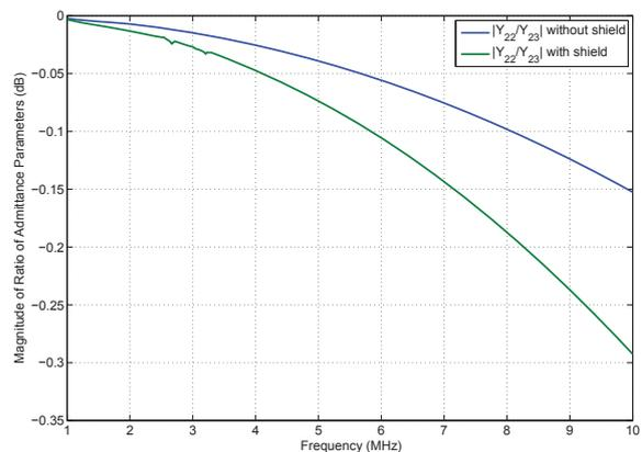
Fig. 24. The magnitude of the ratio  $\frac{Y_{22}}{Y_{23}}$  with and without the shield. As can be seen, the shield does degrade the current balun behavior slightly as the ideal value of this ratio is 0 dB for a current balun. Nevertheless, the degradation is small.
