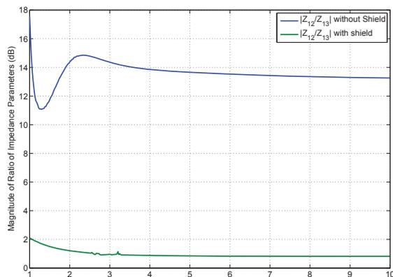
Fig. 22. The magnitude of the ratio  $\frac{Z_{12}}{Z_{13}}$  with and without the shield. As can be seen, the magnitude of the ratio  $\frac{Z_{12}}{Z_{13}}$  is approximately 14 dB without the shield, but is reduced to less than 1 dB with the shield. This simulated data illustrates one of main points of this paper—the shield does little to perturb the short circuit current balance, but dramatically improves open-circuit voltage balance.
