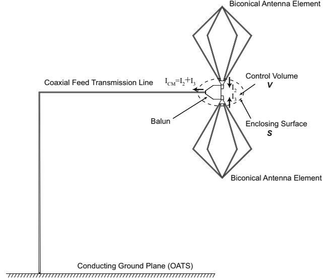
Fig. 4. Biconical antenna in vertical polarization above conducting ground plane. The CM current on the feed transmission line is  $I_{CM} = I_2 + I_3$ .
