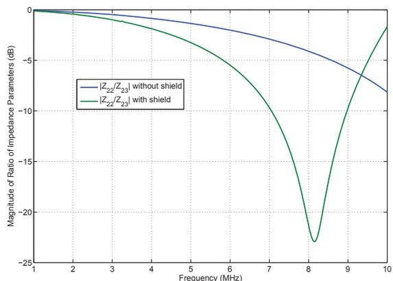
Fig. 25. The magnitude of the ratio  $\frac{Z_{22}}{Z_{23}}$  with and without the shield. The behavior of the magnitude of the ratio of  $\frac{Z_{22}}{Z_{23}}$  is complicated by the unavoidable presence of capacitance to ground even without the shield. Nevertheless the shield changes this ratio markedly and the transformer with a shield cannot serve as a true voltage balun.
