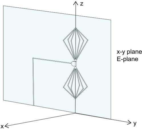
Fig. 9. E-plane of vertically-polarized biconical antenna over ground. Note that the feed transmission line lies completely within the E-plane. The ground plane is the  $x$ - $y$  plane.
