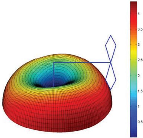
Fig. 13. 3-dimensional radiation pattern depicting the total gain of the vertically-polarized biconical antenna driven by a current balun at 60 MHz.
