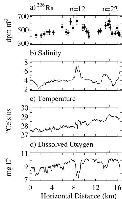
**Figure 3.** Results for a) dissolved  $^{226}\text{Ra}$  (samples 12 and 22 are marked with ticks on all frames), b) surface salinity, c) water temperature, and d) dissolved  $O_2$ . Water temperature and dissolved  $O_2$  generally increased during the course of the day. The influence of the Nueces River is apparent in the low surface salinity and dissolved  $^{226}\text{Ra}$  activity near survey km 15.5; another surface salinity low near km 1.5 may be a plume or eddy of Nueces River water.
