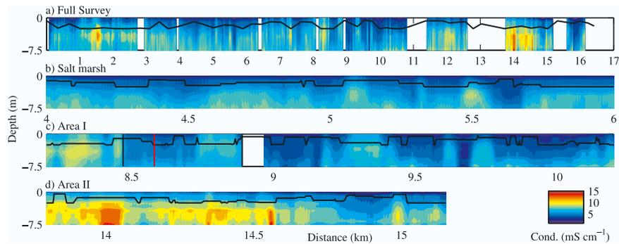
**Figure 2.** Results of the conductivity survey including a) the full survey path; b) a segment along the salt marsh shoreline; c) Area I, west of White's Point, with elevated surface salinity; and d) Area II containing pipeline indications and the Nueces River channel. In c), the location of the surface salinity maxima ( $S > 7$ ) are indicated by vertical black lines and the survey maximum Ra activity (sample 12) by a vertical red line. Water depth is indicated by a black line in all panels.
