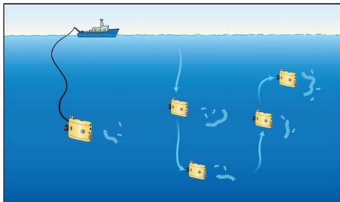
Fig 2. A typical *Mesobot* tracking mission will begin with a teleoperated phase, where the vehicle can be controlled by a human pilot via a tether. After locating a suitable target, the tether will be released and the vehicle will track the target autonomously using its stereo cameras and its control system.
