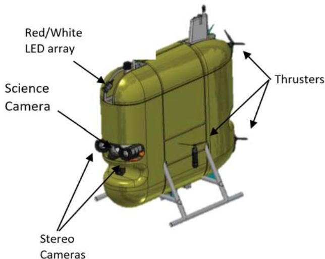
Fig 1. The *Mesobot* will be an autonomous underwater vehicle designed to follow slow-moving midwater targets such as zooplankton, fish, and particle aggregates. The vehicle will carry stereo cameras for target tracking and a high-quality video/still camera for scientific documentation. It will use a combination of thrusters and a variable buoyancy system for maneuvering. The *Mesobot* will be 1.5 meters tall and displace approximately 200 kg.
