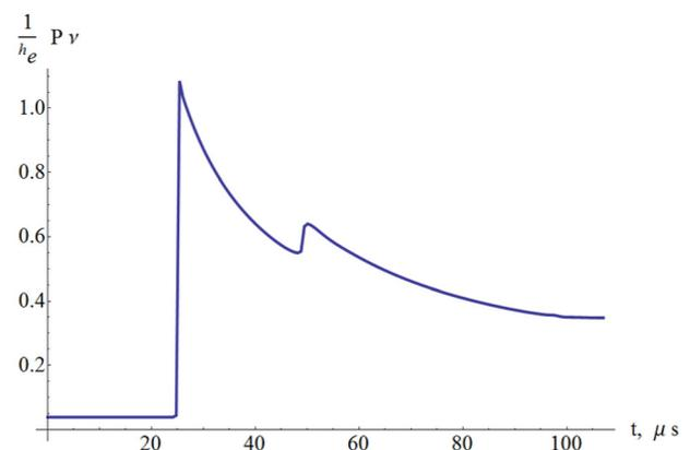
FIG. 5. Time dependence of the dimensionless  $\frac{1}{h_e} P \nu$  at the base of a closed cylindrical reactor. Here  $P$ ,  $\nu$  is pressure and specific volume per unit mass at the reactor base,  $h_e = 2.12$  MJ/kg is the reaction energy per unit mass.
