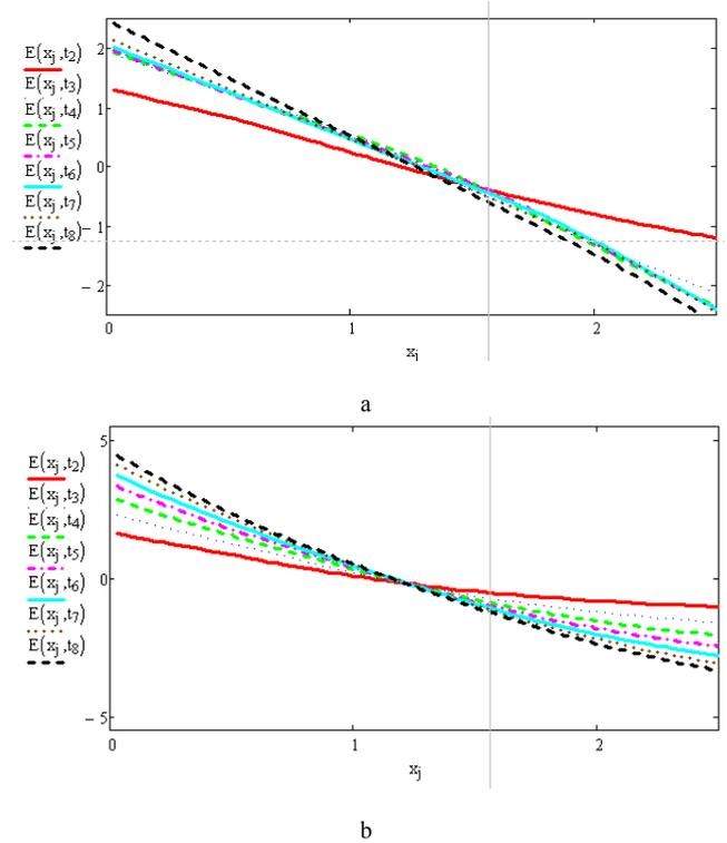
**Figure 8.** (a) - Computation neglecting the gravity: the distribution the electric field intensity along the sample axis at subsequent time moments; (b) - Gravity acts oppositely to the thermal wave propagation  $G = -100$ ,  $\alpha_R = 0$ ,  $\beta_R = 100$ .
