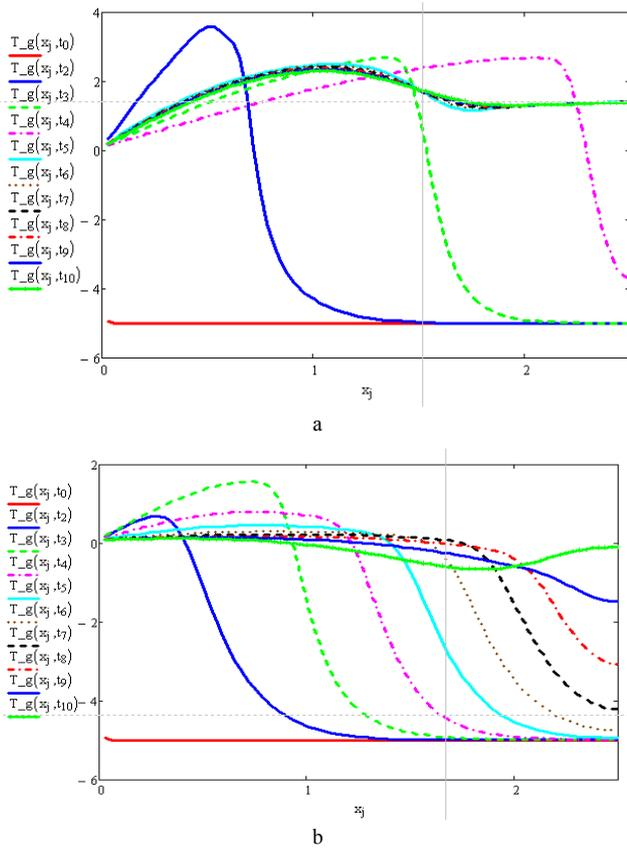
**Figure 2.** (a) - The gravity effect on temperature distribution along the sample at subsequent moments. Gravity is co directional to the thermal wave propagation (from the left side to the right side)  $G=100, \alpha_R=0, \beta_R=100$ ; (b) - The temperature distribution along the sample at subsequent moments with the neglected gravity.
