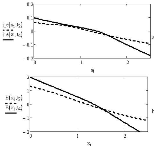
**Figure 7.** Computation neglecting the Gravity: (a) - Distribution of the electric field Intensity ( $E$ ) along the sample at the moments  $t_2 = 12$ , (dashed line) and  $t_4 = 24$  (solid line); (b) - The current density distribution along the sample at the moments  $t_2 = 12$ , (dashed line) and  $t_4 = 24$  (solid line)
