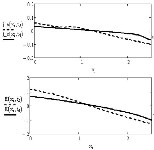
**Figure 6.** Gravity force acts coincidentally to the thermal wave propagation (from the left side to the right side)  $G = 100$ ,  $\alpha_R = 0$ ,  $\beta_R = 100$ . (a) - Distribution of the electric field Intensity ( $E$ ) along the sample at the moments  $t_2 = 12$ , (dashed line) and  $t_4 = 24$  (solid line). (b) - The current density distribution along the sample at the moments  $t_2 = 12$ , (dashed line) and  $t_4 = 24$  (solid line).
