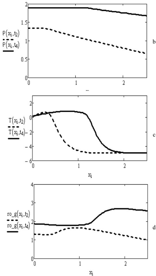
**Figure 4.** Computation neglecting the gravity: (a) - Distribution of the sulfur ions velocity along the sample at moments  $t_2, t_4$ ;  $t_4 > t_2$ ; (b) - The vapors pressure along the sample at the moments  $(t_2, t_4)$   $t_2=12$  (dashed line),  $t_4=24$  (solid line); (c) - Distribution of the temperature along the sample at moments  $t_2, t_4$ ;  $t_4 > t_2$ ; (d) - The vapors density along the sample at the moments  $(t_2, t_4)$   $t_2=12$  (dashed line),  $t_4=24$  (solid line)
