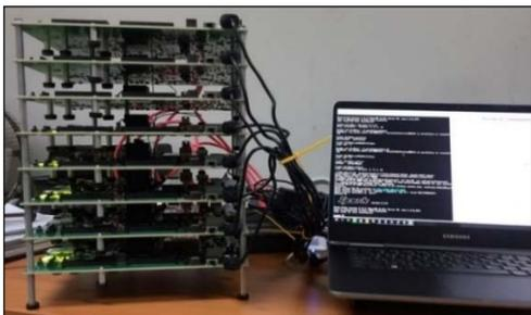
Fig 4. Cluster prototype with eight Zynq UltraScale+ boards
