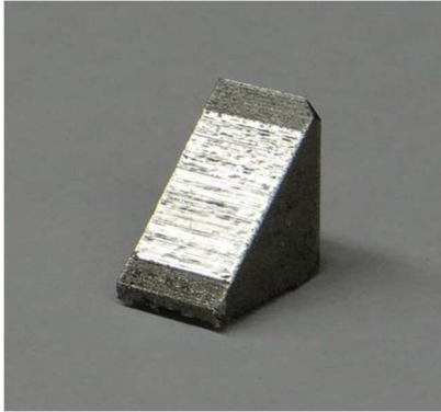
Fig. 4 Inclined SLM manufactured sample after applying SLR process
