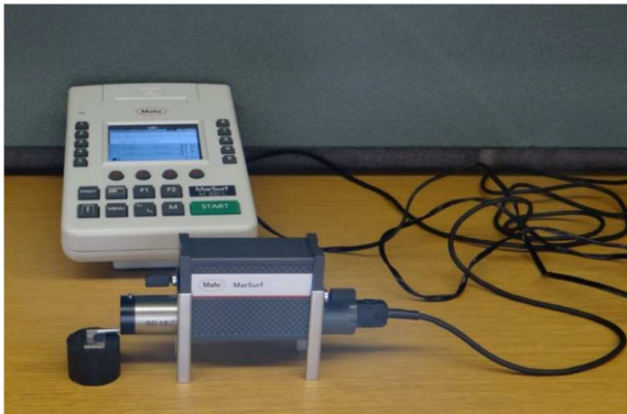
Fig. 5 Roughness measuring instrument set up
