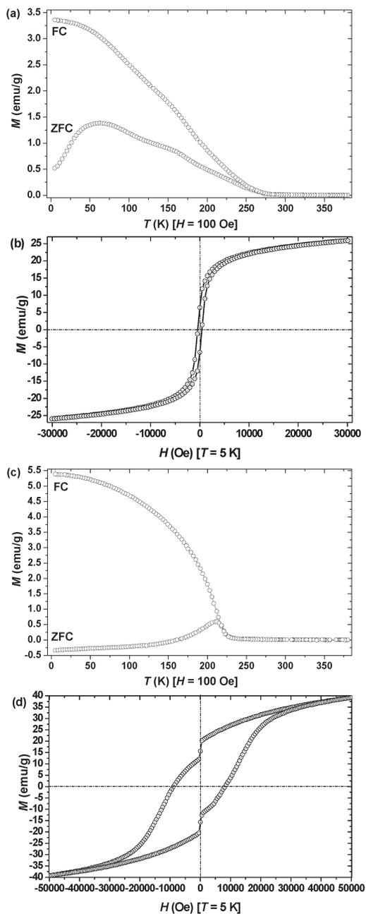
**Fig. 5** (a) Temperature dependences of zero-field-cooled and field-cooled magnetization of LNMO nanoparticles in an applied field of 100 Oe. (b) Field-dependent magnetization data at 5 K of LNMO nanoparticles. (c) Temperature dependences of zero-field-cooled and field-cooled magnetization of LCMO nanoparticles in an applied field of 100 Oe. (d) Field-dependent magnetization data at 5 K of LCMO nanoparticles.
