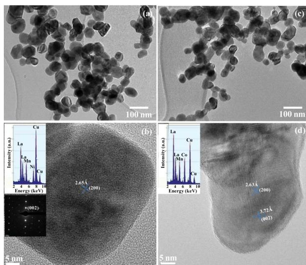
**Fig. 4** Typical low magnification TEM images of the as-synthesized (a) LNMO and (c) LCMO nanoparticles. HRTEM images of the (b) LNMO and (d) LCMO nanoparticles with corresponding EDX (the Cu peaks originate from the TEM grid) as well as SAED of LNMO.
