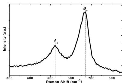
**Fig. 2** Raman spectrum of the as-synthesized LNMO nanoparticles.
