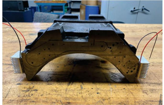
Figure 4: Bearing Adapter with mounted TEGs
