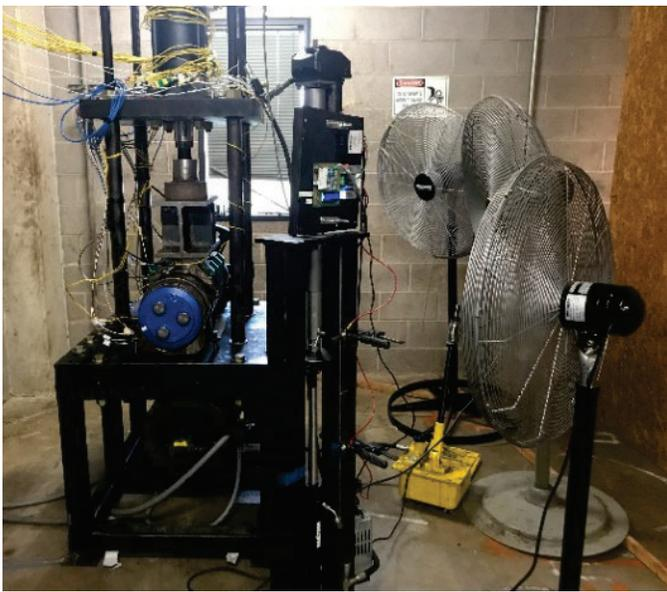
Figure 3: Four Bearing Tester (4BT)
