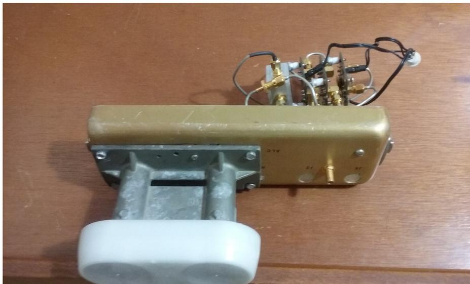
Figure 9: Frontal view of the transmitting horn
