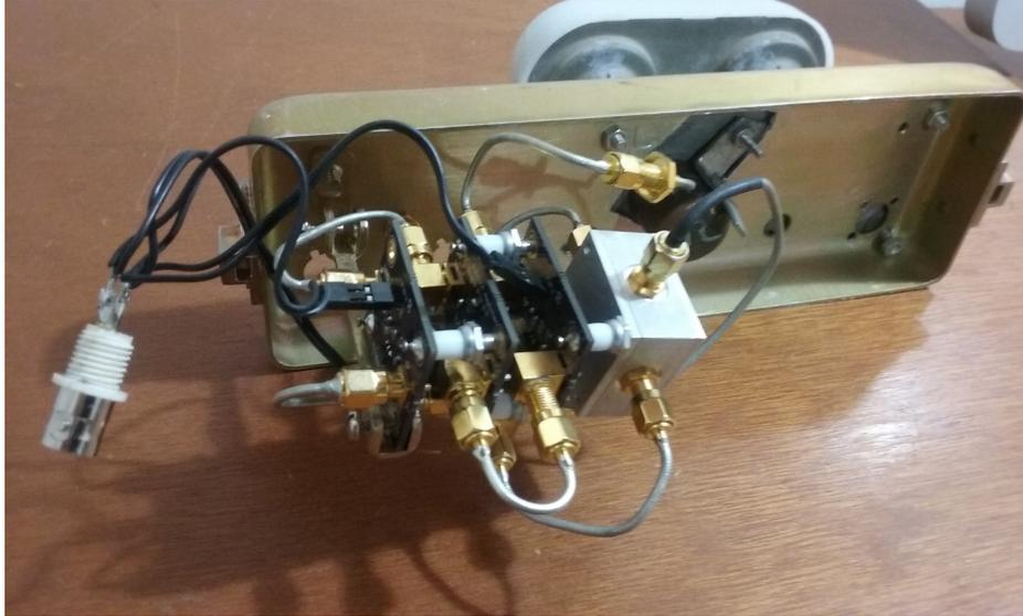
Figure 8: The frequency multiplier mounted on the transmit horn
