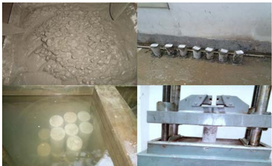
Figure 3. Concrete mix, casting, curing and compressive strength test in UTM.
