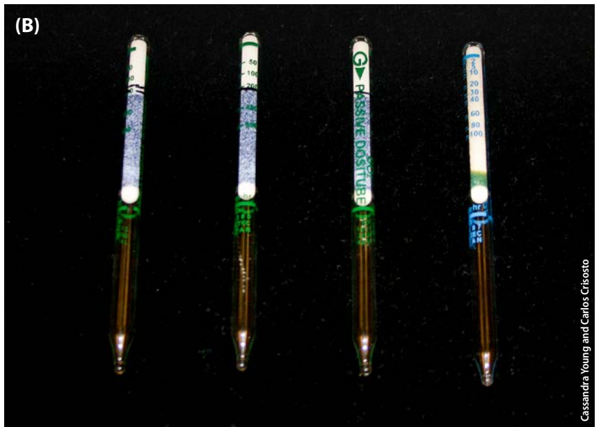
FIG. 2. (A) Mycelial growth of C. cladosporioides , C. limoniforme and C. ramotenellum in lidded petri plates treated with SO 2 of 0, 100, 200 or 400 ppm-h. (B) Passive colorimetric dosimeter tubes were used to measure SO 2 concentrations. (C) One was placed inside each fumigation chamber, opposite the SO 2 input valve.
