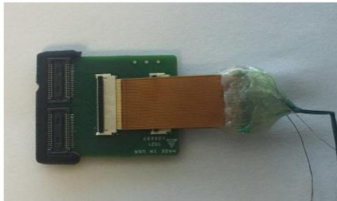
Figure 2.10: Ribbon cables connected to the TDT 128-channel interface board connector
