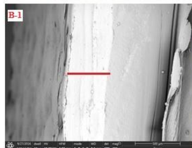
B-1 Cross-sectional view (Thickness 505 \pm 10 \mu\text{m} )
