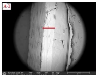
A-1 Cross-sectional view (Thickness 461 \pm 15.6 \mu\text{m} )
