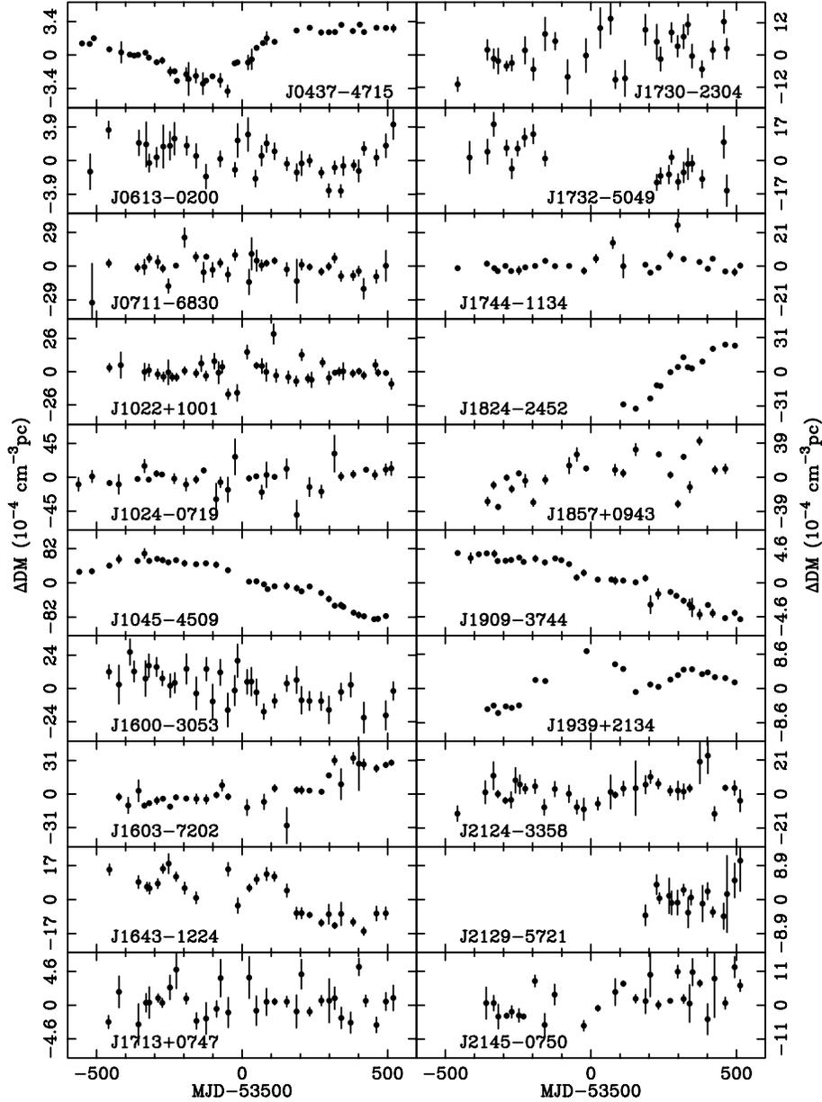
**Figure 2.** DM variations of 20-ms pulsars. Note a  $\Delta\text{DM}$  of  $10^{-4} \text{ cm}^{-3} \text{ pc}$  corresponds to time delays at 10 cm of 43 ns, at 20 cm of 212 ns and at 50 cm of 884 ns.
