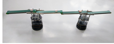
Fig. 1: A robot chain formed by two mobile conveyors.
