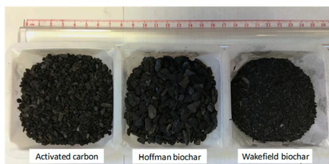
**Figure 2.** Pyrogenic carbon materials tested in this study.
