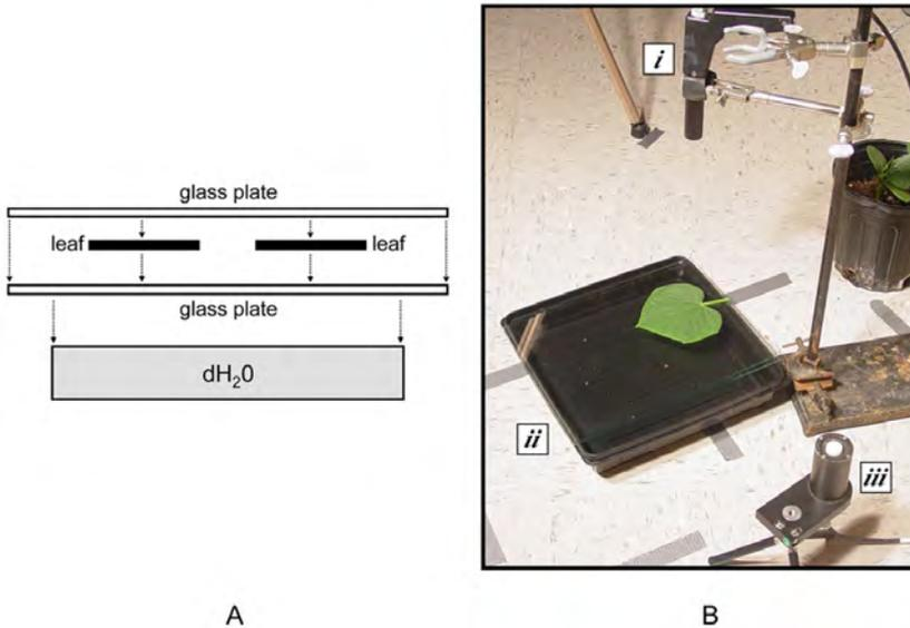
Fig. 4. Diagram of the *in situ* image acquisition template used to examine individual leaves acquired from healthy and stressed whole plants (A). Photo of the image acquisition template demonstrating the use of the [i] VNIR sensor, [ii] glass plates, and [iii] remote cosine receptor used to collect spectrophotometric data (B). A CIR camera may be mounted at the same level as the spectroradiometer VNIR sensor shown above [i].
