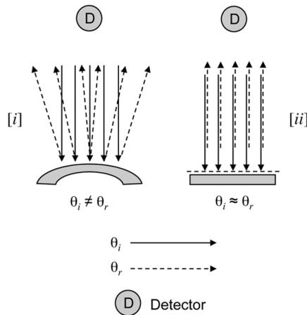
Fig. 3. Reduction of light scattering [i] results when leaves exhibiting synclastic Gaussian curvature are compressed [ii]. Compression of the leaves using the *in situ* image acquisition template results in light reflected at angles ( $\theta_r$ ) equivalent or nearly so to incident light ( $\theta_i$ ), which improves the quality of sample detection via image acquisition or spectroradiometry.
