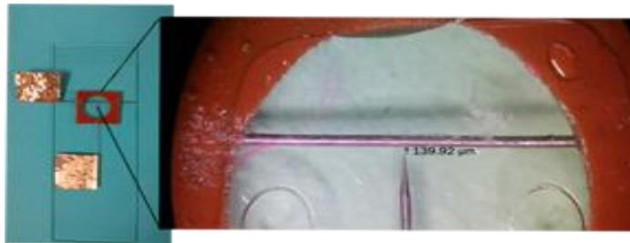
**Figure 6:** Orthogonal electrode pair on a PDMS coated glass slide
