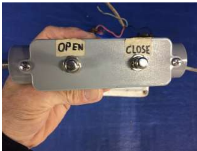
Fig. 11 Control for shutter
