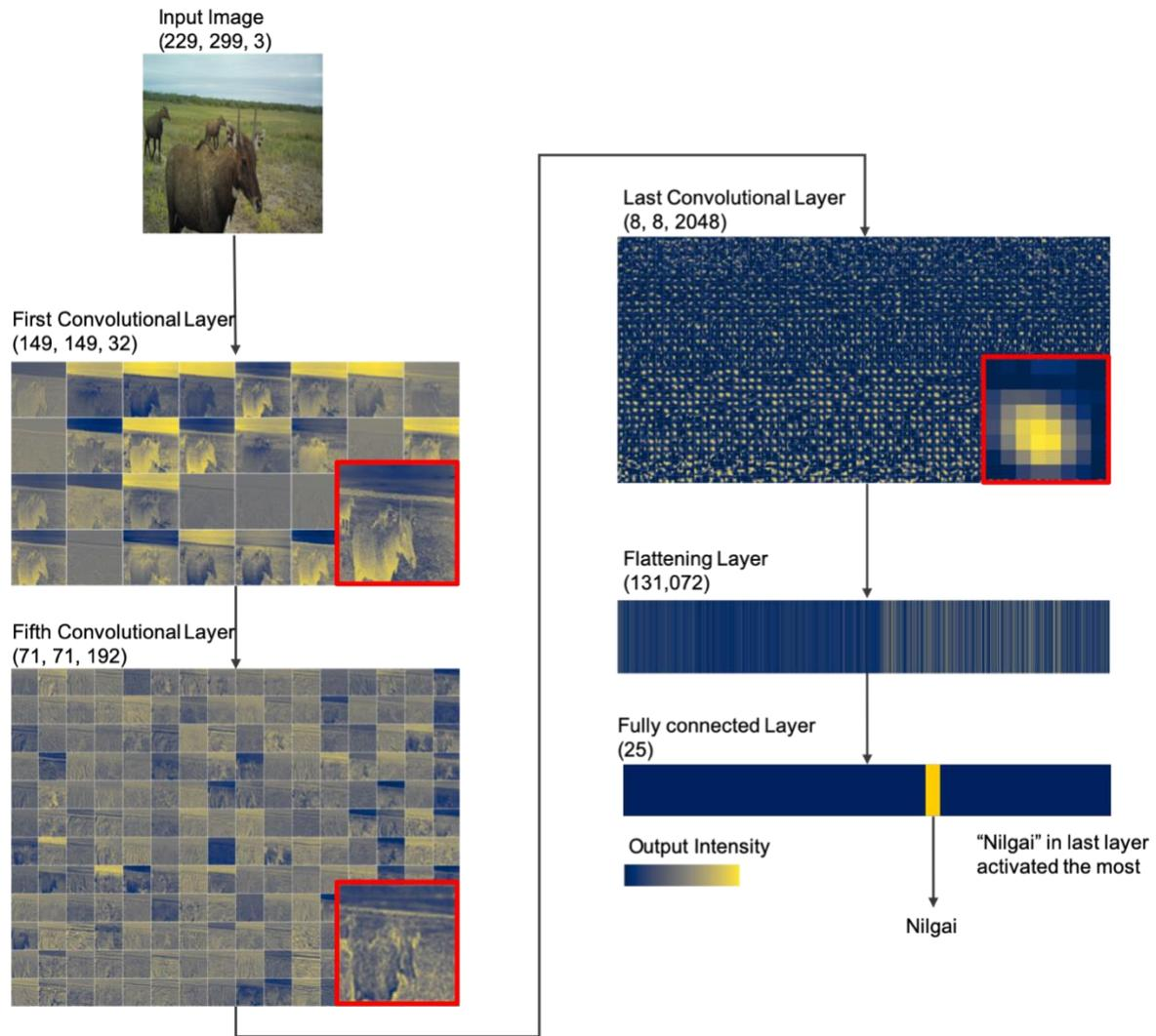
Figure 3.2 Inside A Convolutional Neural Network
