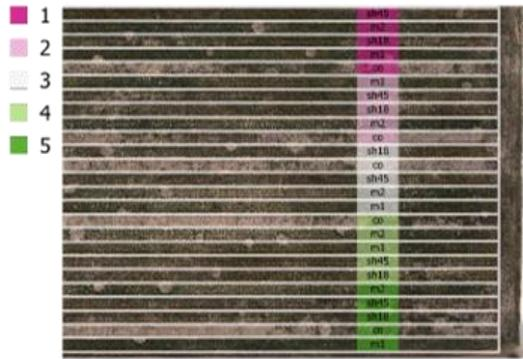
a) Six-band ortho-mosaic constructed and treatment design.
