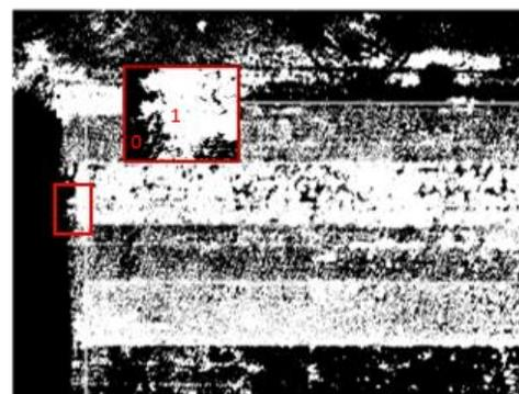
d) Binary image was created using NDVI thresholding value of 0.4 that delineated vegetation (1) and non-vegetation (0).
