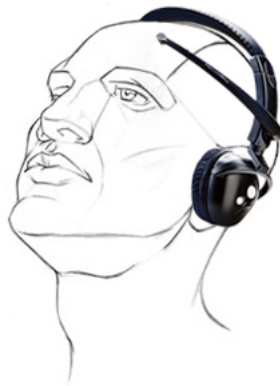
Figure 4.1: EEG MindSet's electrode placed on forehead (modified from reference [23]).
