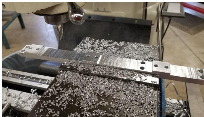
Figure 4.2. – Aluminum Piece, Manufactured On A Milling Machine.
