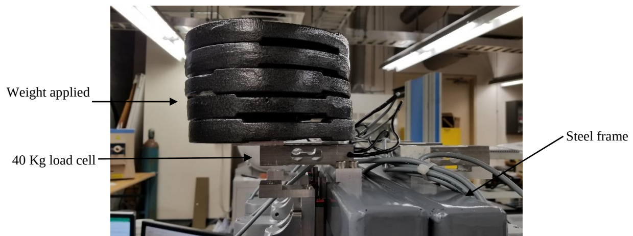
Figure 4.16. – Load Applied To A Load Cell For Calibration.
