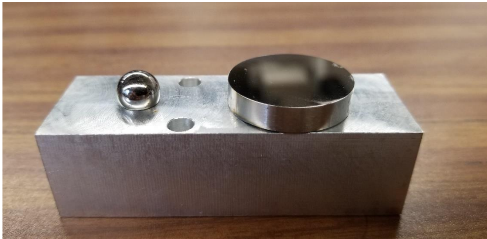
Figure 4.20. Cocrmo Alloy Disc And Steel Ball Used During The Wear Tests.
