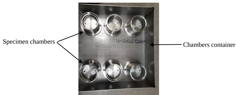
Figure 4.8. – Specimen Chambers Mounted On The Chambers Container.
