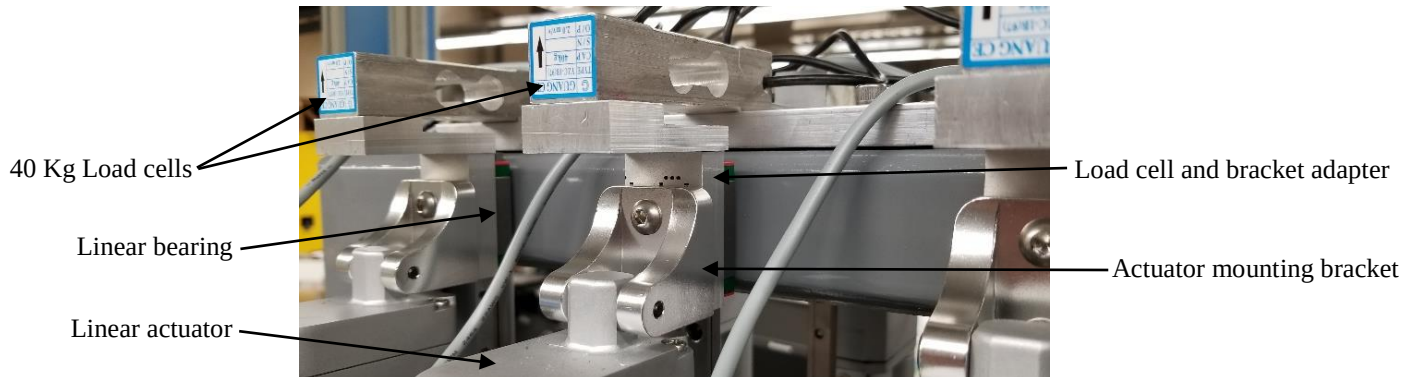
Figure 4.9. – Load Cell Mounted Above The Linear Actuator.
