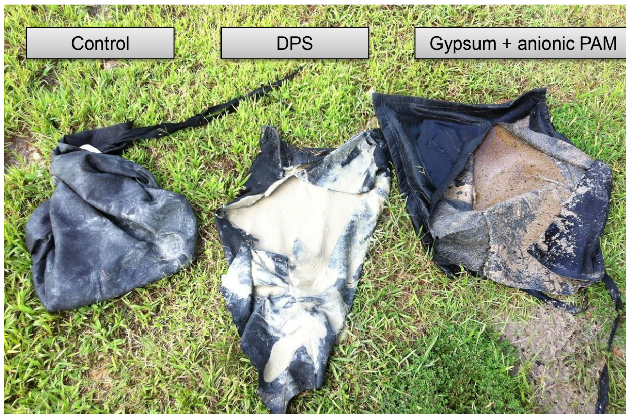
Fig. 7 Inside of dewatering bags after pumped water tests.
