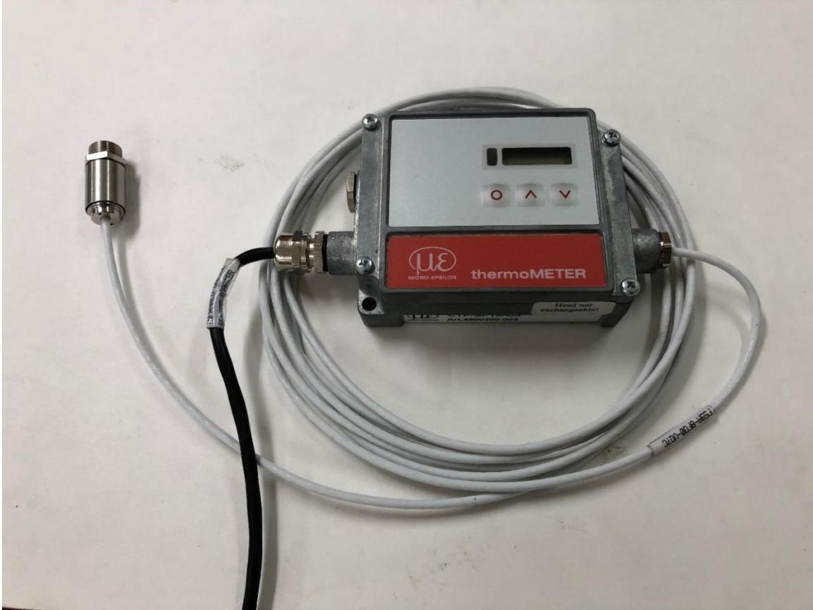
Figure 16. MICRO-EPSILON infrared (IR) temperature sensor
