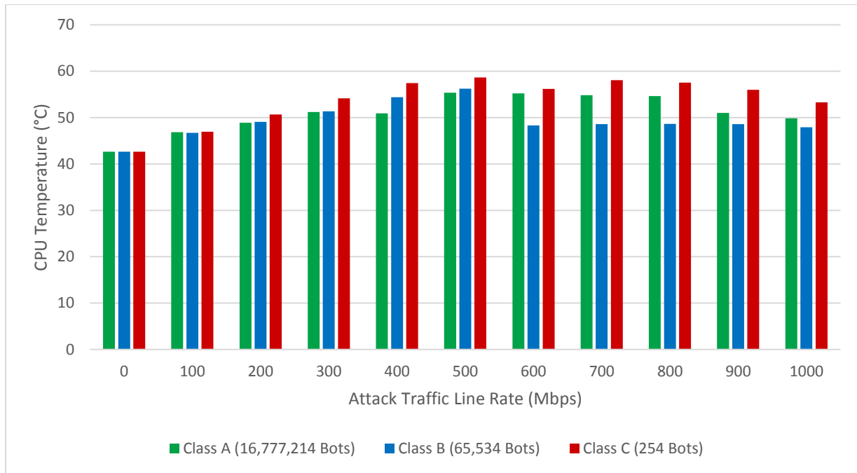
Figure 4.7 CPU Temperature under Ping Attacks on macOS High Sierra
