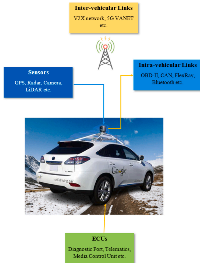
Fig. 1. Basic components of an autonomous vehicle.
