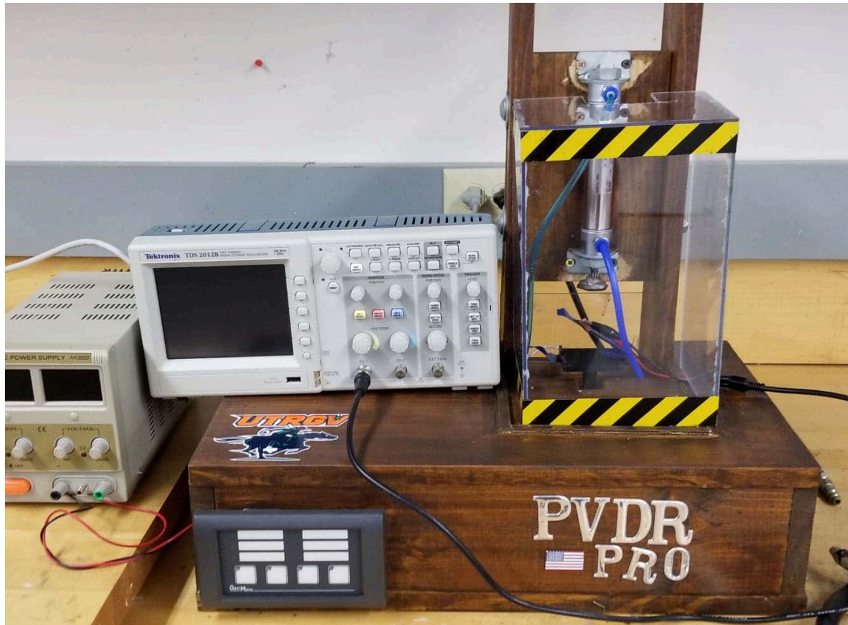
Figure 14: PVDR-Pro and Oscilloscope set up for piezoelectric testing
