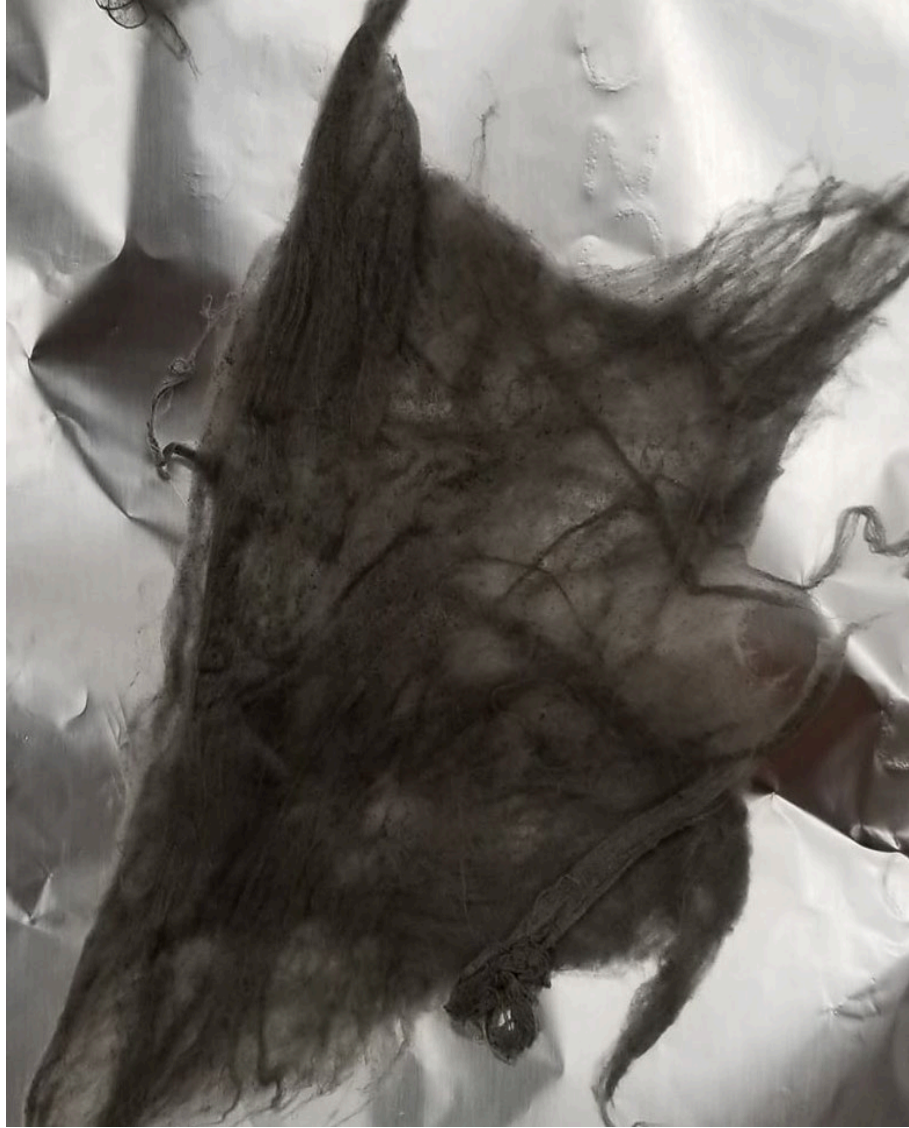
Figure 30: PVDF-PPy doped fiber sample
