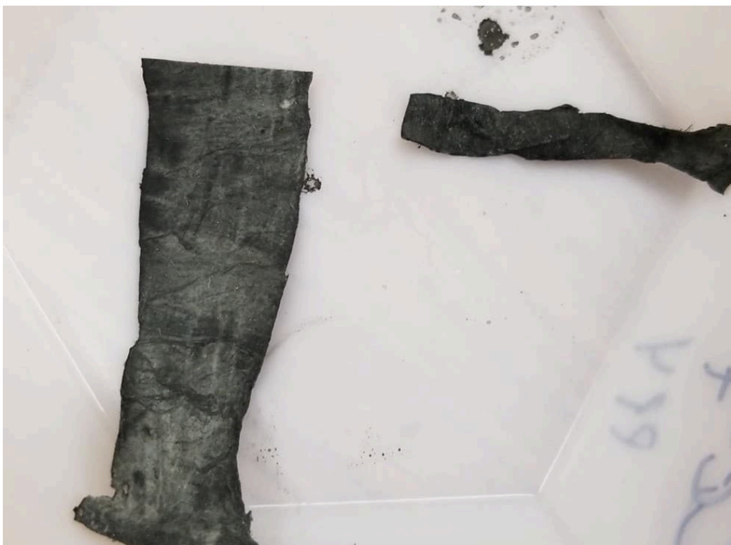
Figure 29: Coating method 7. Fiber samples after coating
