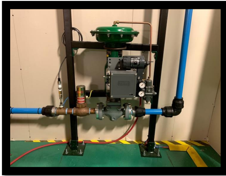
Figure 33: Pressure valve system
