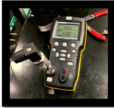
Figure 19: PX313 calibration on PCL819 device
