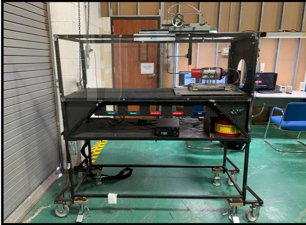
Figure 16: Jet Turbine Test Stand (JTTS)
