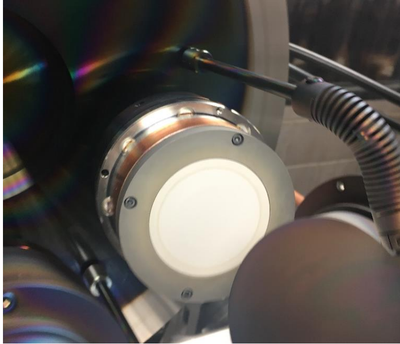
Figure 4.4 - h-BN target mounted in the RF gun of the MSS
