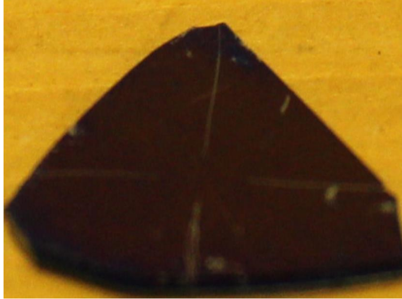
Figure 5.7 - cBN thin film ( \approx 900 nm thickness) on Si 100 substrate with cut insulating channels for required thin-film geometry.
