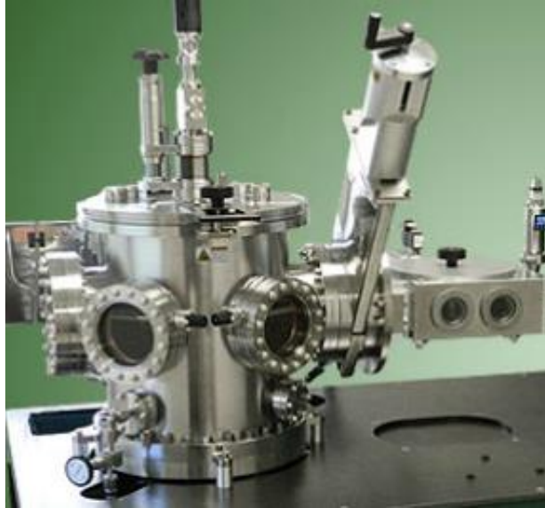
Figure 4.1 - Ultra High Vacuum (Main) Chamber and Load Lock Chamber with Gate Valve and glass windows
