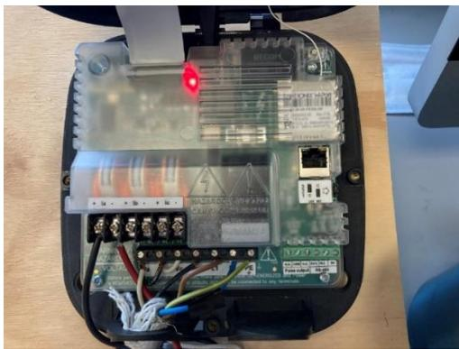
*Figure 71. EPM 6100 Internal Circuit.*
