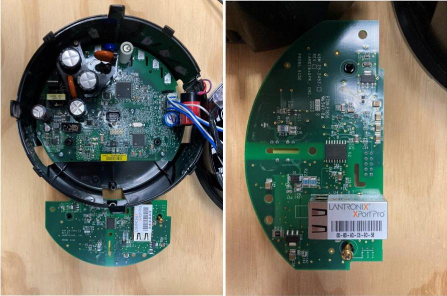
Figure 69. (Left) Metrology module and communication module from a S4x Ethernet meter disassembled. (Right) S4x Ethernet communication module.
