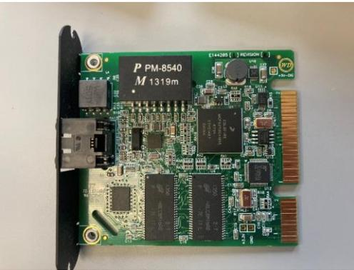
*Figure 73. EPM 7000's network interface card.*
