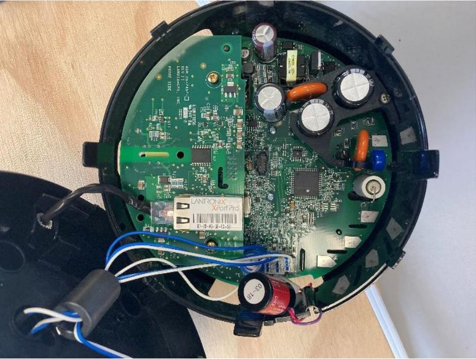
Figure 65. S4x Ethernet internal circuitry.
