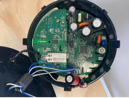
*Figure 72. S4x Ethernet internal circuit.*
