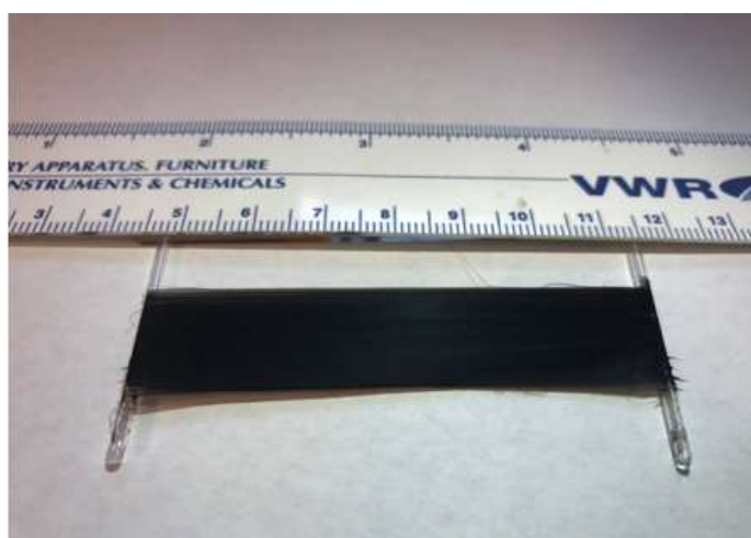
Figure 2.2: Multi-walled carbon nanotubes sheet extracted from carbon nanoforest.
