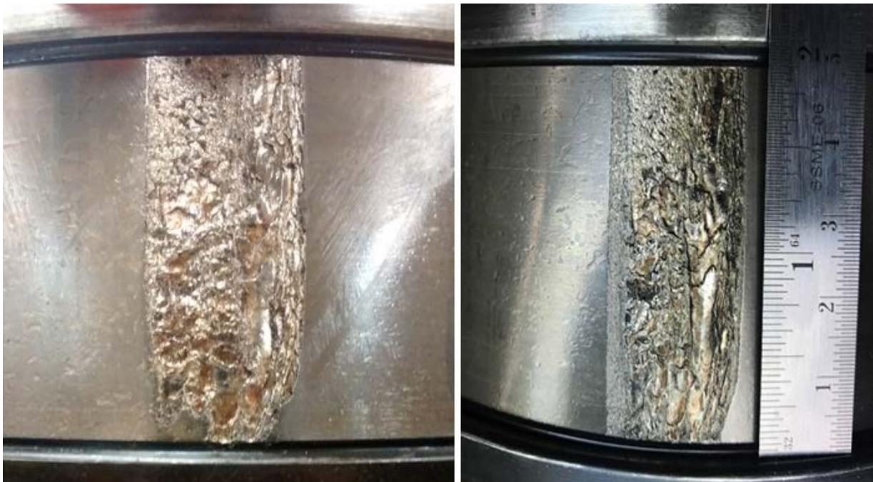
Figure 36. Experiment 202A: Initial cone raceway (left) and final cone raceway (right)
