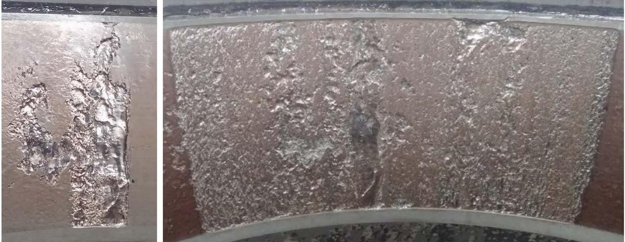
Figure 33. Experiment 184B: Initial cup raceway (left) and final cup raceway (right)
