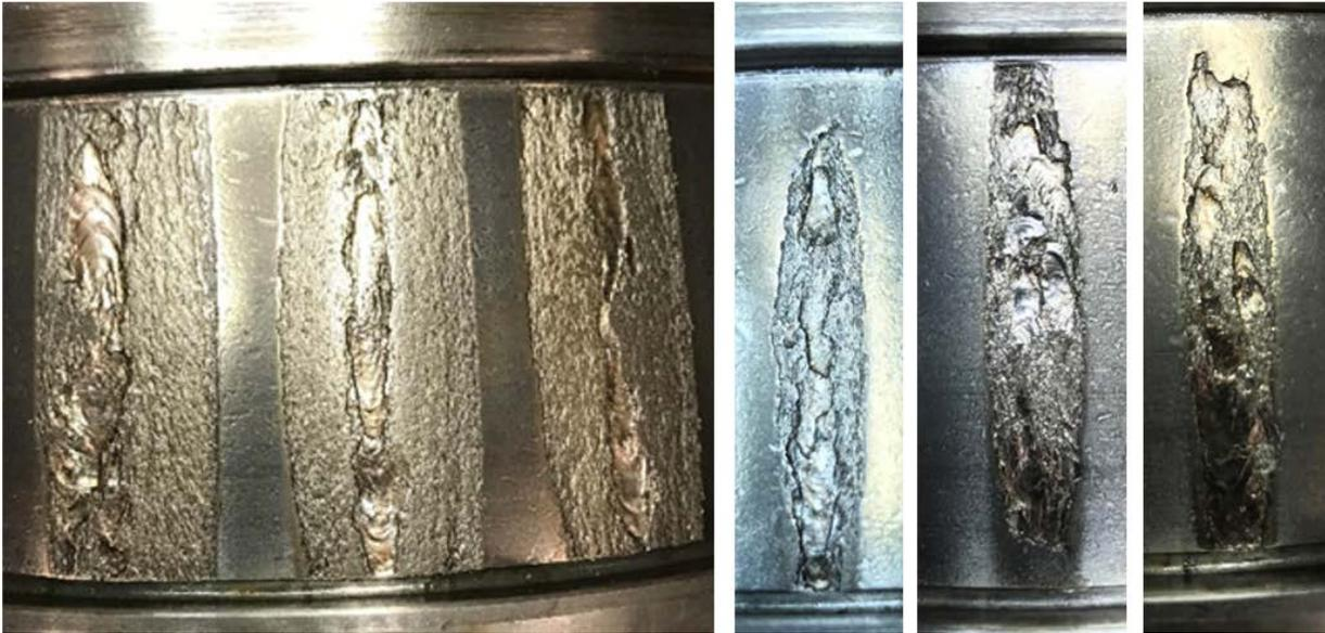
Figure 40. Experiment 206 final cone raceway
