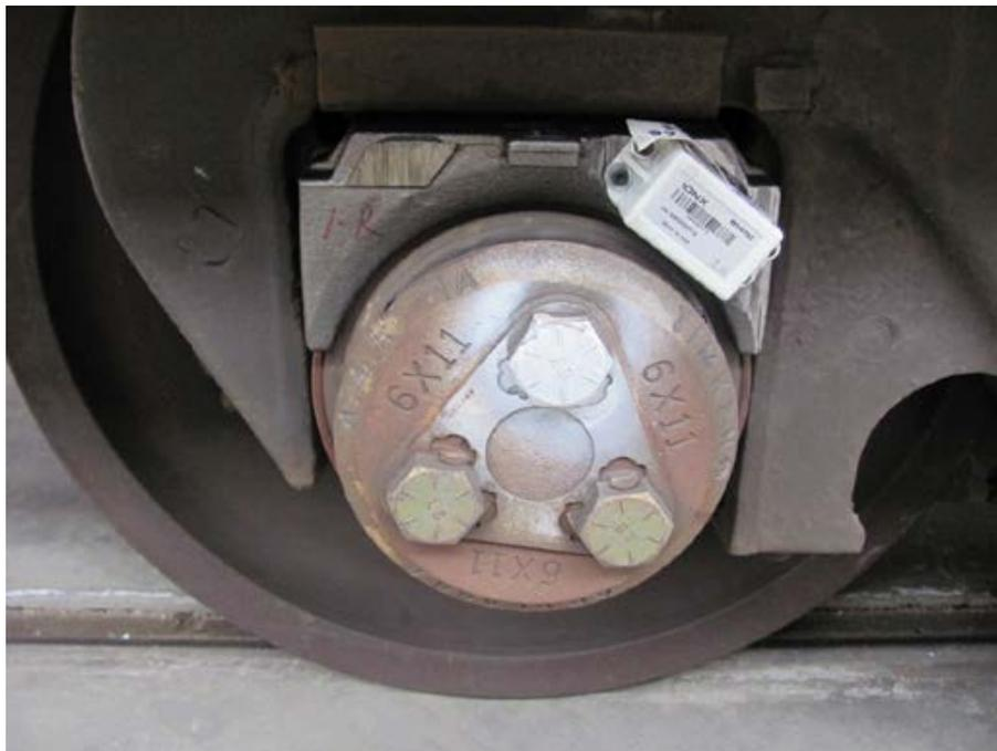
Figure 7. Field installation of a Wireless Sensor Node
