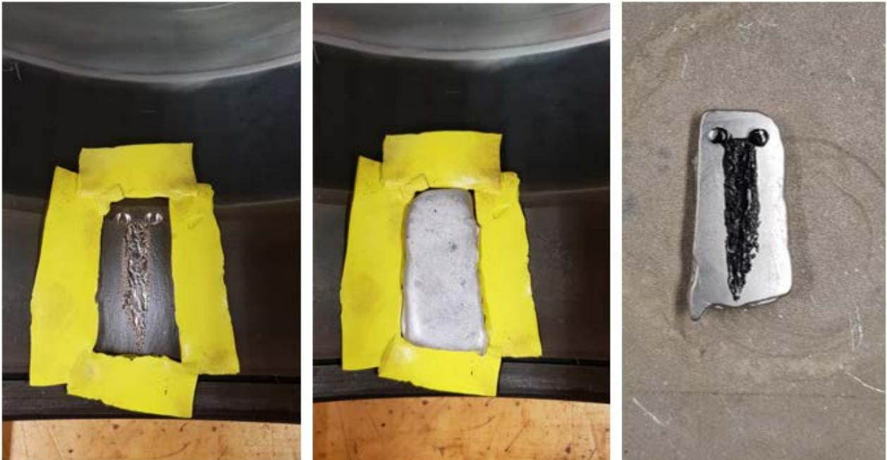
Figure 17. Casting procedure using sealant and bismuth tape
