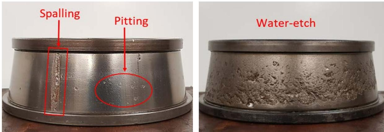
Figure 3. Example of localized defects (left) and distributed defect (right)
