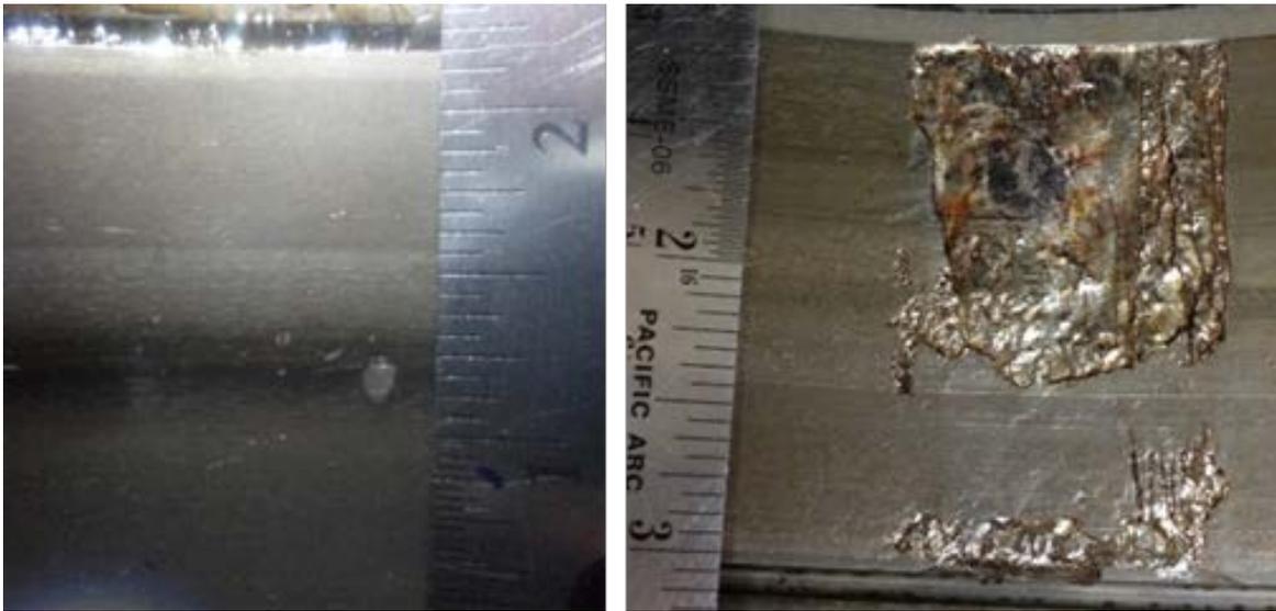
Figure 30. Experiment 200: Initial cup raceway (left) and final cup raceway (right)
