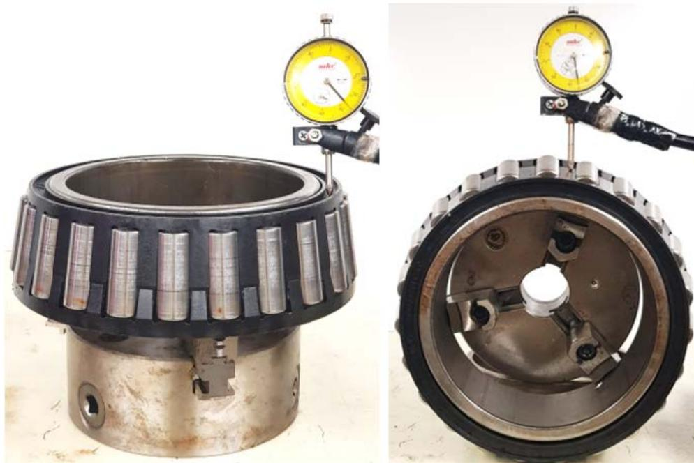
Figure 8. Cage measurement set-up: cage lift (left), cage shake (right)
