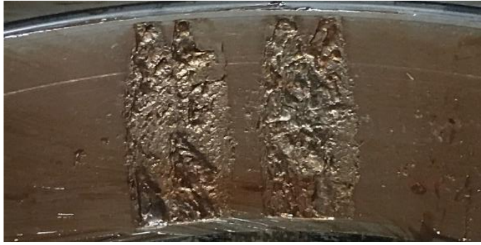
Figure 19: Bearing 2 (B2) cup spall Spall 1 (left): Area = 1.575 \text{ in}^2 ; Spall 2 (right): Area = 1.546 \text{ in}^2
