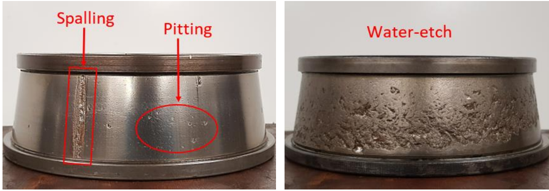
Figure 4. Example of localized defects (left) and distributed defect (right)
