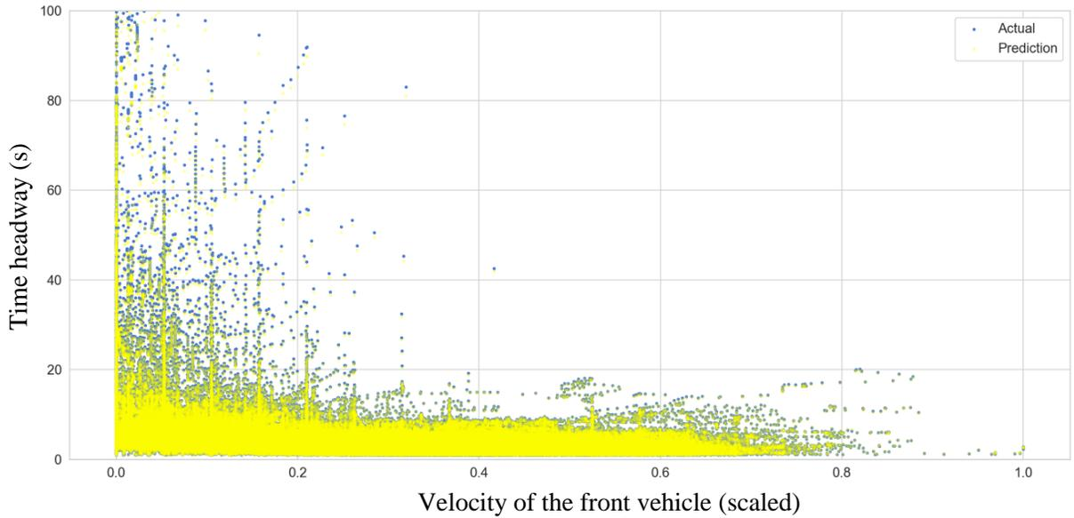
Figure 33. Correlation of Preceding (front vehicle) velocity with time headway in US-101 (actual vs predicted)
