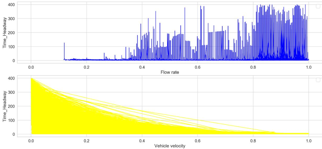
Figure 9. Correlation of time headway with flow rates and velocity
