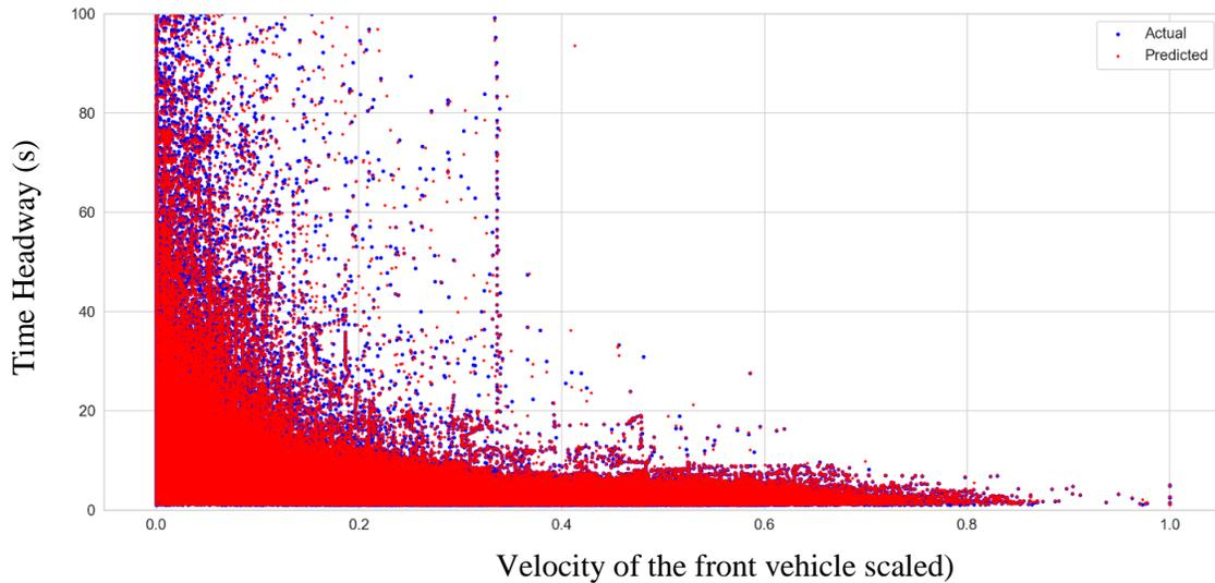
Figure 32. Correlation of Preceding (front vehicle) velocity with time headway in I-80 (actual vs predicted)
