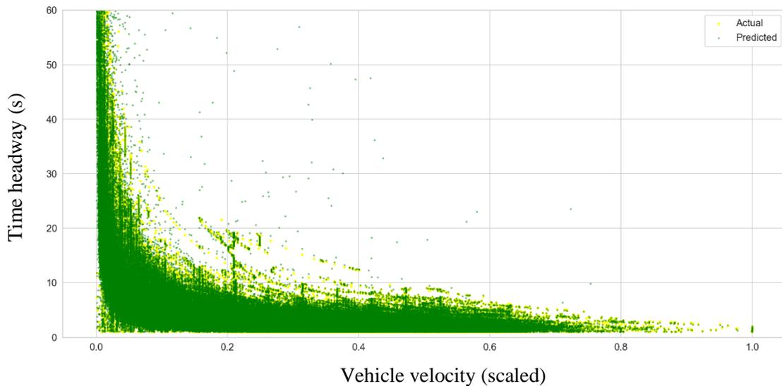
Figure 30. Correlation of vehicle velocity with time headway in I-80 (actual vs predicted)
