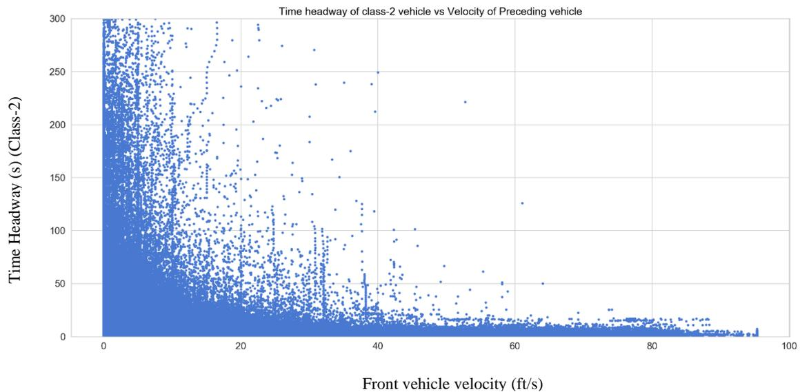
Figure 16. Effect of the velocity of preceding vehicle on Passenger Cars
