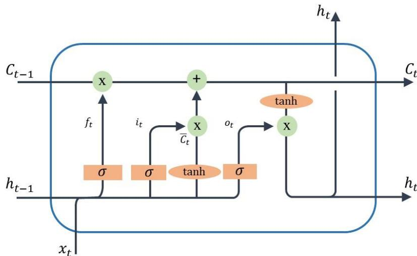
Figure 2. Unit LSTM cell
