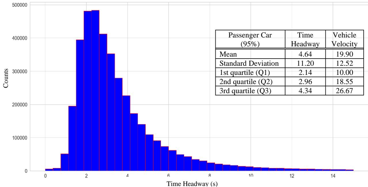
Figure 12 Time Headway distribution of Vehicle Class-2 (Passenger Car)
