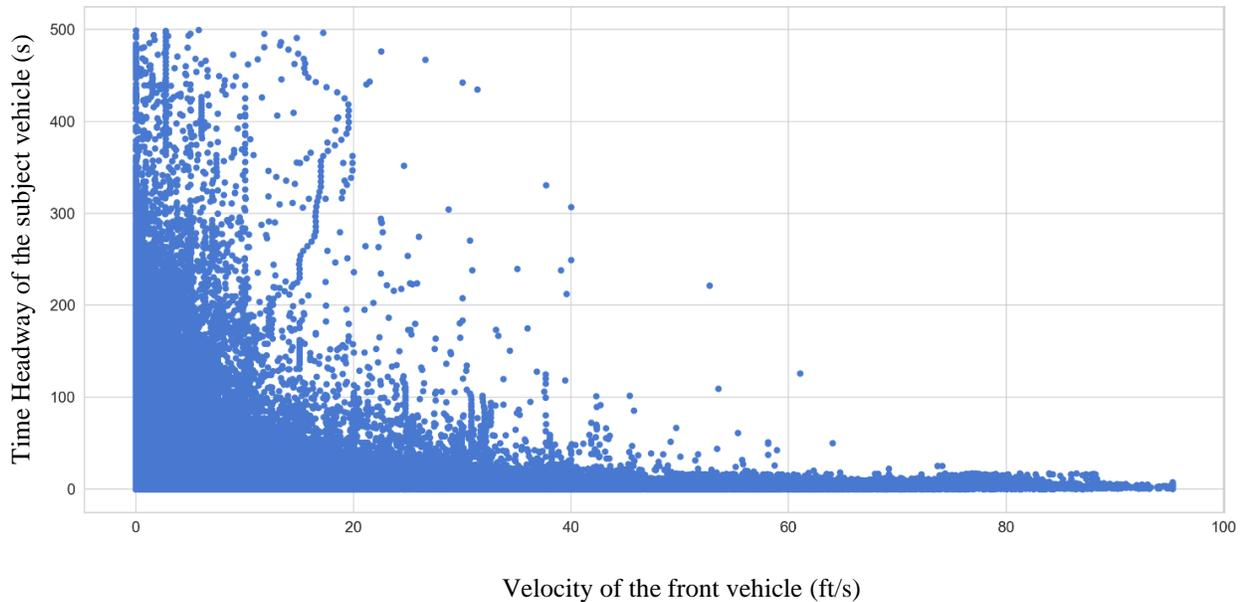
Figure 8 Velocity of preceding vehicle vs Time headway of subject vehicle
