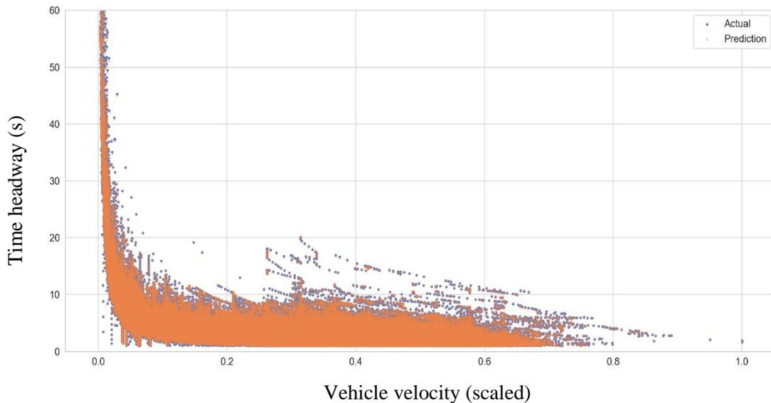
Figure 31. Correlation of vehicle velocity with time headway in US-101 (actual vs predicted)
