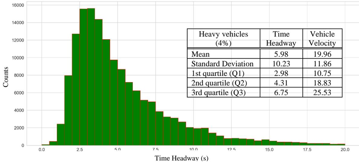
Figure 13. Time Headway distribution of Vehicle Class-3 (truck)
