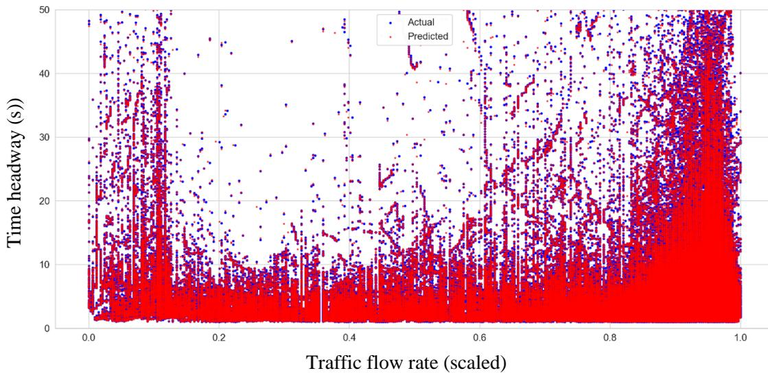
Figure 34. Correlation of time headway (actual vs predicted) with flow rate in highway I-80
