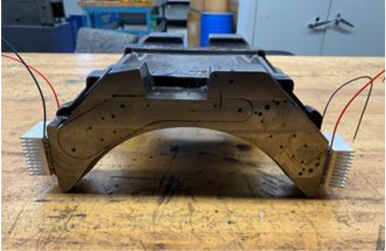
Figure 4. TEG/Heat sinks mounted on the bearing adapter
