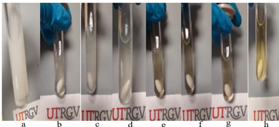
Figure. 3.8: Describes crude product at various DBU concentration for a) 0%, b) 0.50%, c) 1.10%, d) 2.25%, e) 4.34%, f) 6.19%, g) 7.39% and h) 10.14%
