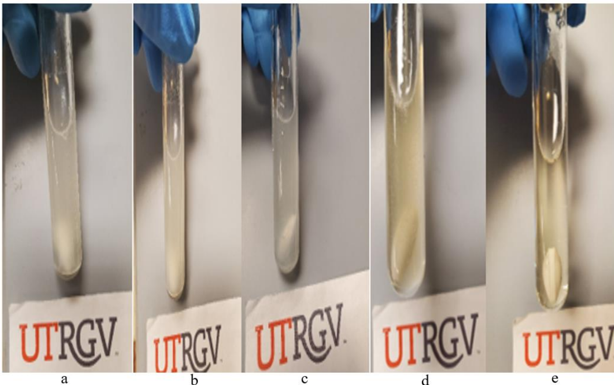
Figure 3.10: Describes the glycolytic product after depolymerization with TBD at a) 180°C , b) 190°C , c) 200°C , d) 210°C, and e) 220°C.
