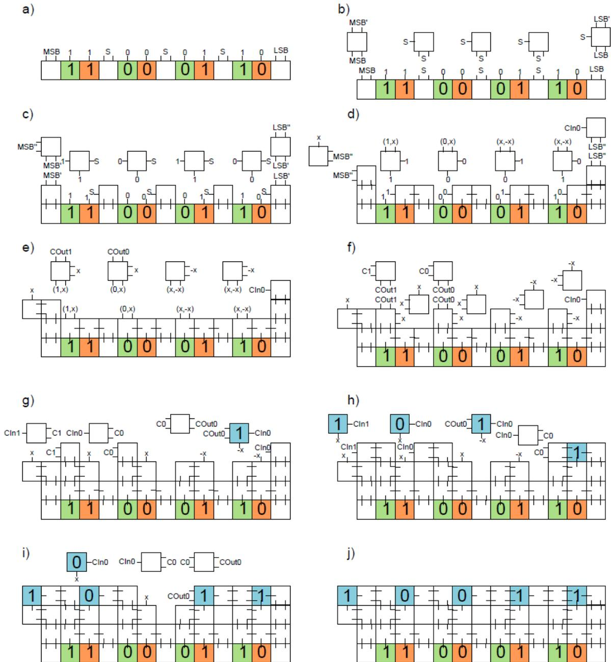
Figure 14 Example of  $O(\log n)$  average case addition  $1001+1010=10011$
