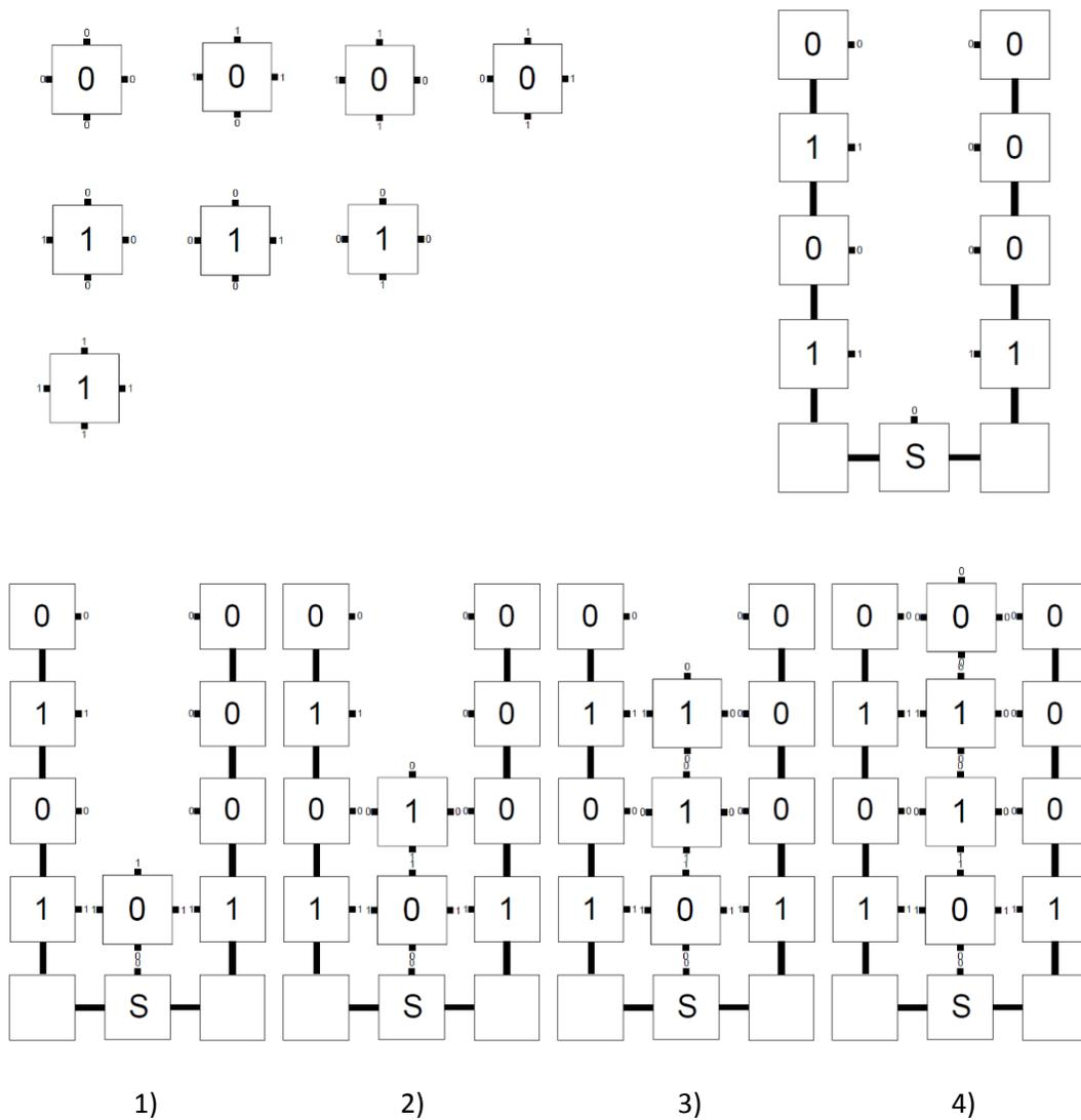
Figure 5 Four steps of adding two numbers. This example shows  $101+1=110$
