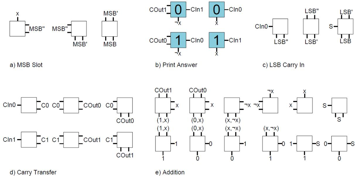
Figure 13 Tile set for implement the average case  $O(\log n)$  runtime and worst case  $O(n)$  runtime addition
