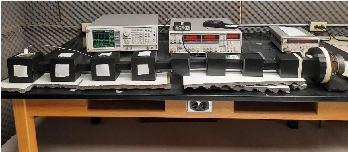
Figure 3. 2: Experimental set up for tunable acoustic filter with the realistic model built using 3d printer.
