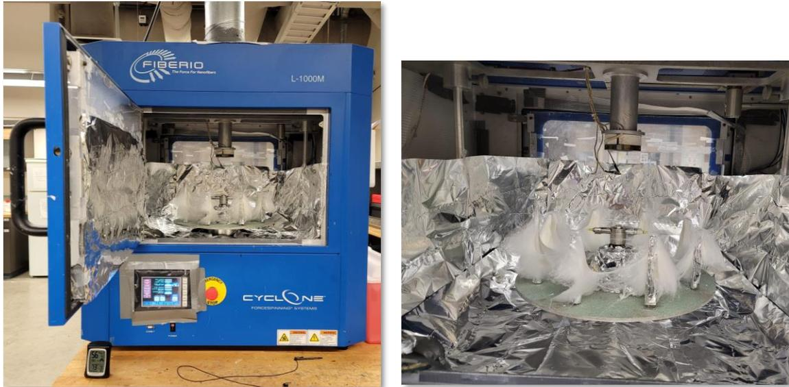
**Figure 5.** Forcespinning cyclone with spun fibers.
