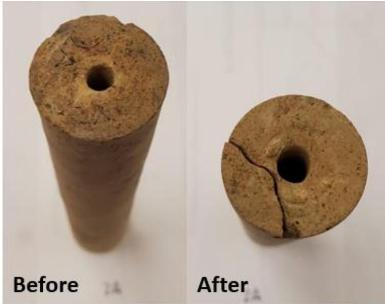
Figure 34. Thru-hole sample before and after acidizing
