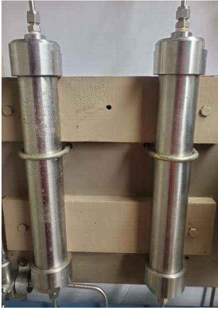
Figure 9. Acid and brine accumulators
