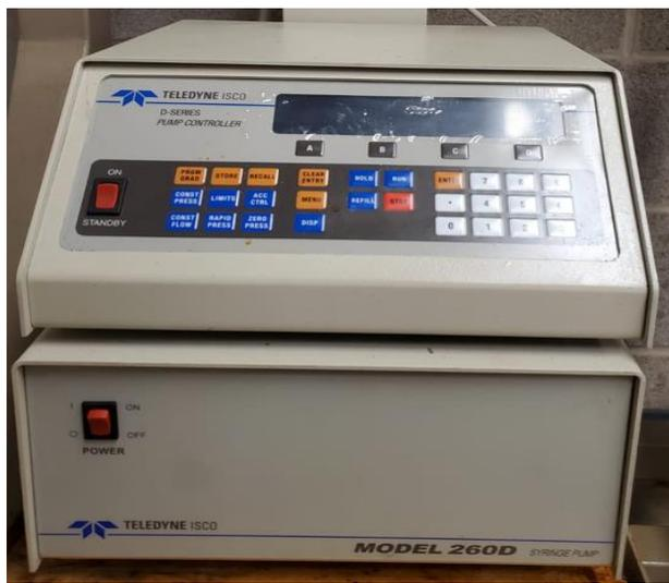
Figure 7. Teledyne ISCO 260D syringe pump
