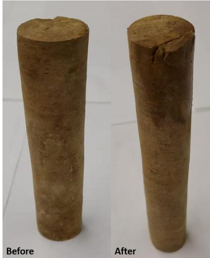
Figure 29. Acid injection in low permeability limestone
