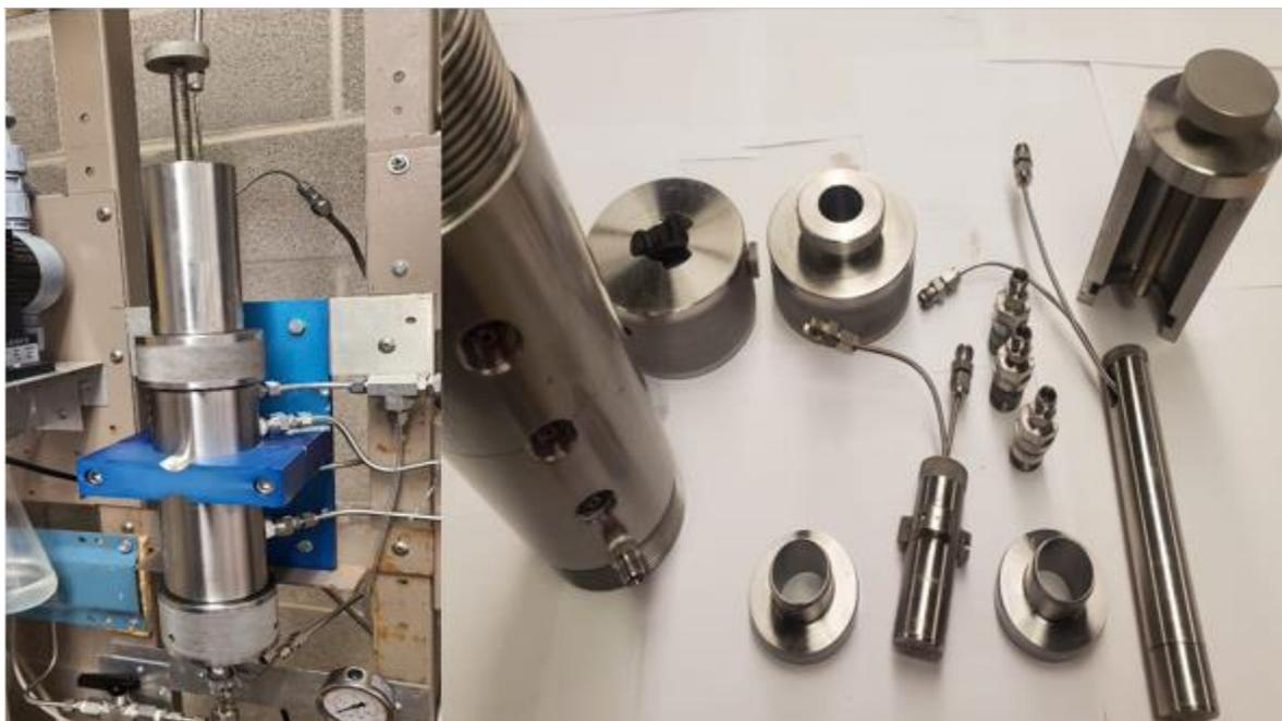
Figure 6. Core Holder assembly and components
