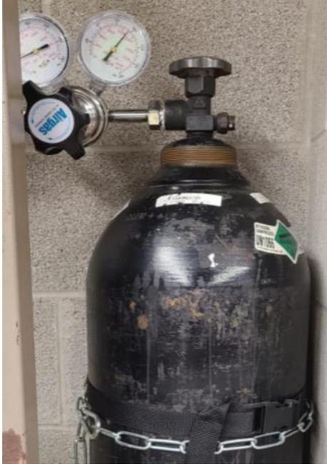
Figure 19. Nitrogen tank and regulator
