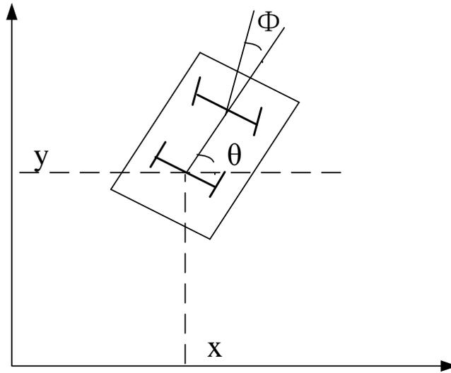
Figure 4.3 Simplified model of four-wheeled car
