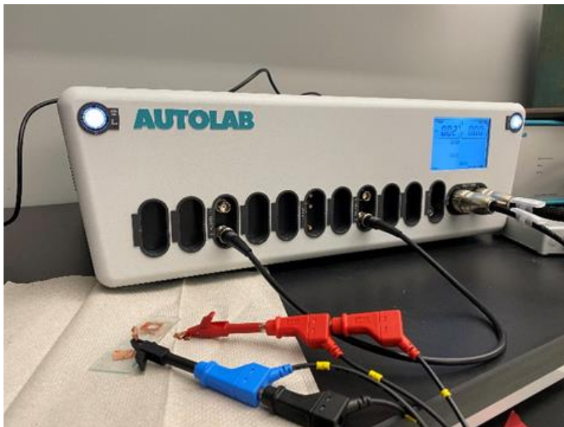
Figure 4.1: Set up of the T electrode in the Autolab potentiostat/galvanostat (AUTO LAB PGSTAT302N)
