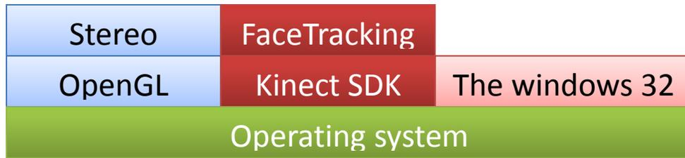
Figure 3 The GPS-MIV Software Architecture
