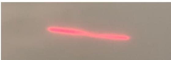
Figure 14: The rotation of the galvo mirrors created a straight-line movement of the point laser.
