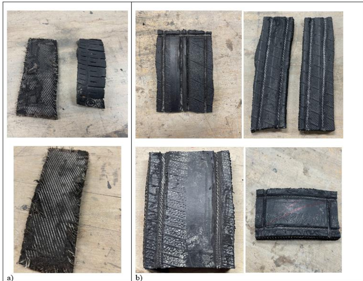
Figure 17: a) Exposed rubber sample. b) Grooved rubber sample.
