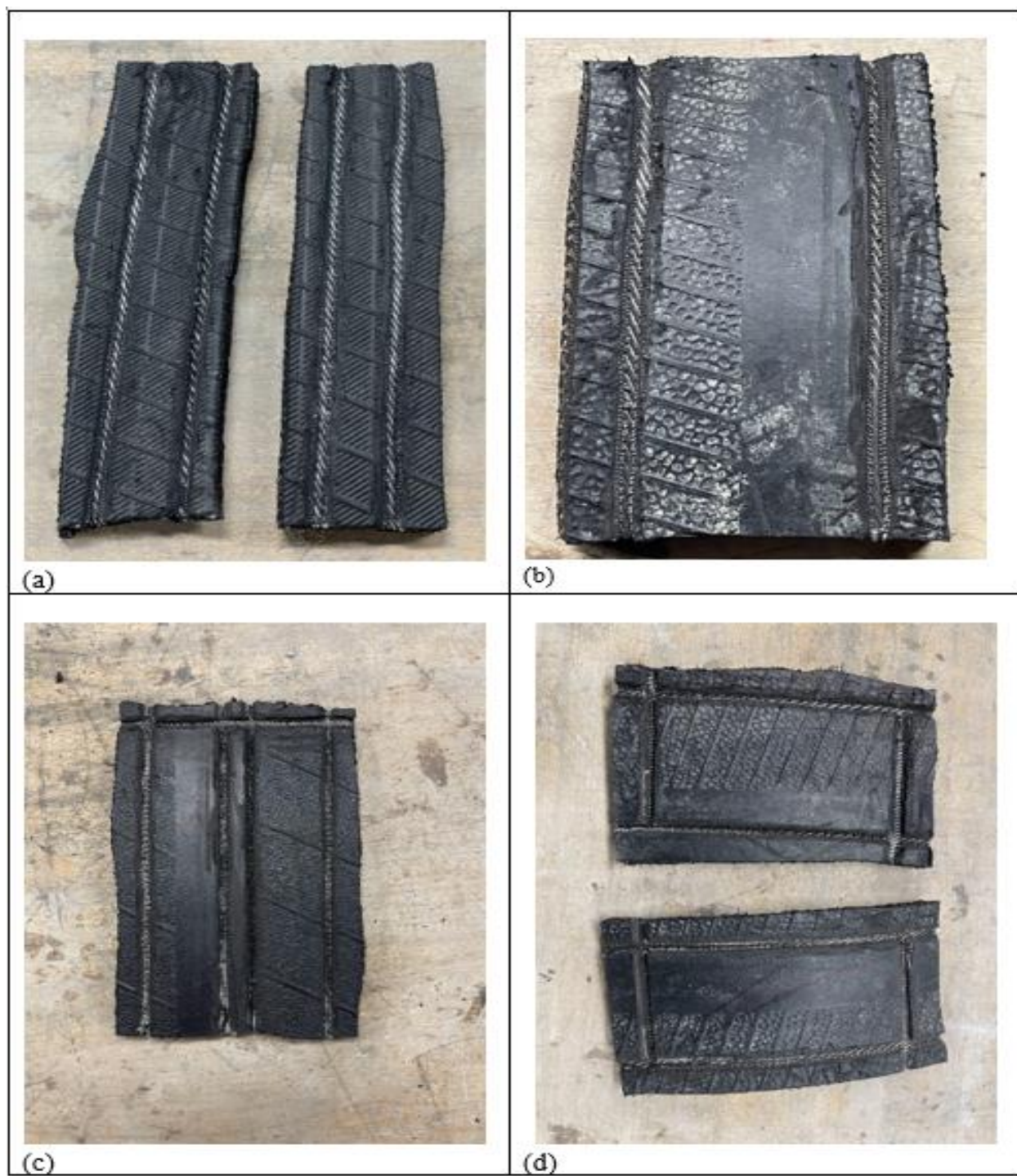
Figure 19: Rubber samples with longitudinal grooves.
