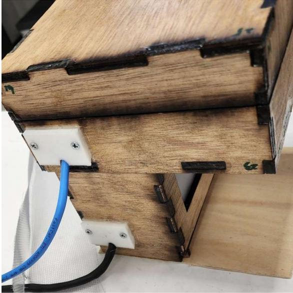
Figure 2.15: Side View of the container with cable lids attached
