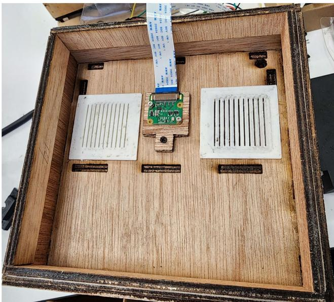
Figure 2.18: Raspberry Pi Camera V2.1 in monitoring system
